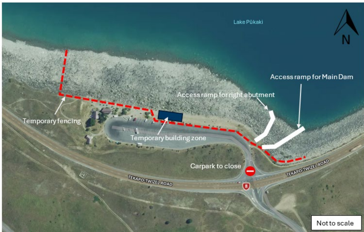
Figure 10 Dam and right abutment - security fencing, closed access, access ramps and temporary buildings
