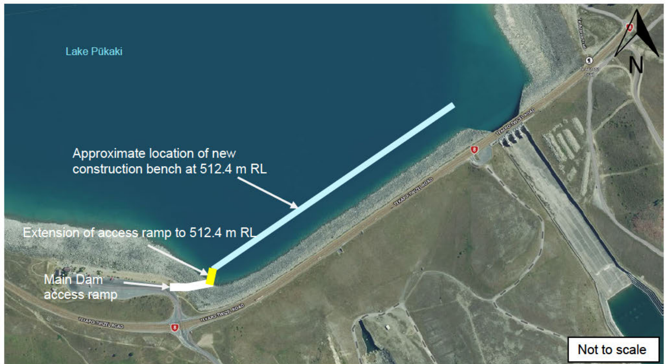
Figure 24 Site plan (Main Dam) and indicative 512.4 m RL construction bench
