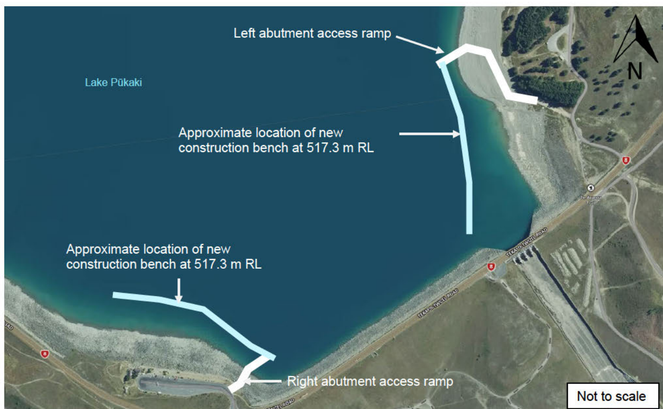
Figure 20 Site plan (abutments) and indicative 517.3 m RL construction bench
