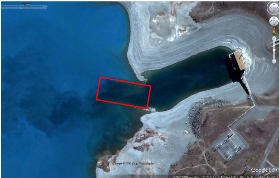
Figure 1.3: Aerial view from Google Earth of Tekapo B Power Station tailrace channel showing outline of submerged weir and rock chute structure (marked by red box)
