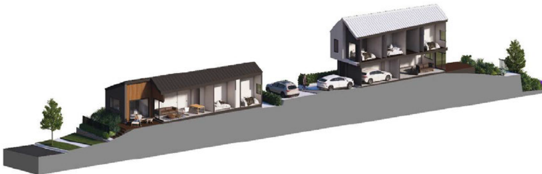
Figure 4 - Cross section showing a dwelling with its rear yard adjoining a public road. A keystone wall is used to define the property boundary while the 1:3 planted slope is used to make up for the difference in height.
