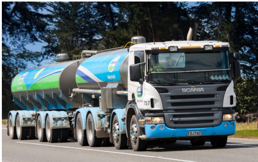
Figure 33 – A large truck and trailer tanker unit, as used by Fonterra to transport milk. These can hold up to 28.8m 3
