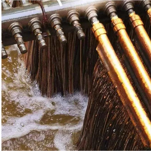
Figure 10 - Hollow Fibre Membranes with visible fouling
