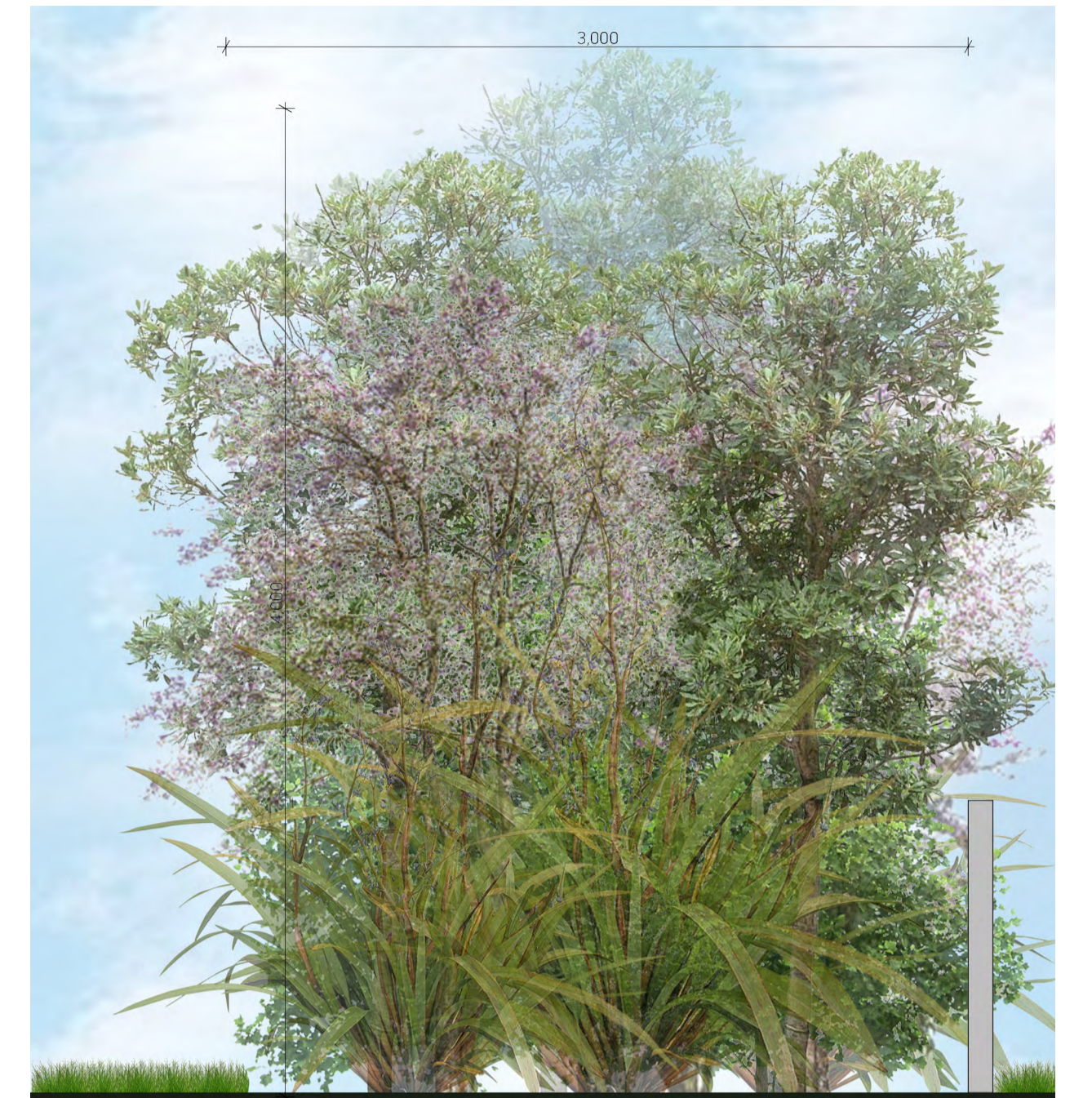
OPTION 1 - TYPICAL SECTION: 3.0m WIDE BUFFER 1:25@A1 / 1:50@A3 Note: Planting shown at 10-year maturity (expected maturity to be achieved at 5 - 7 years)
