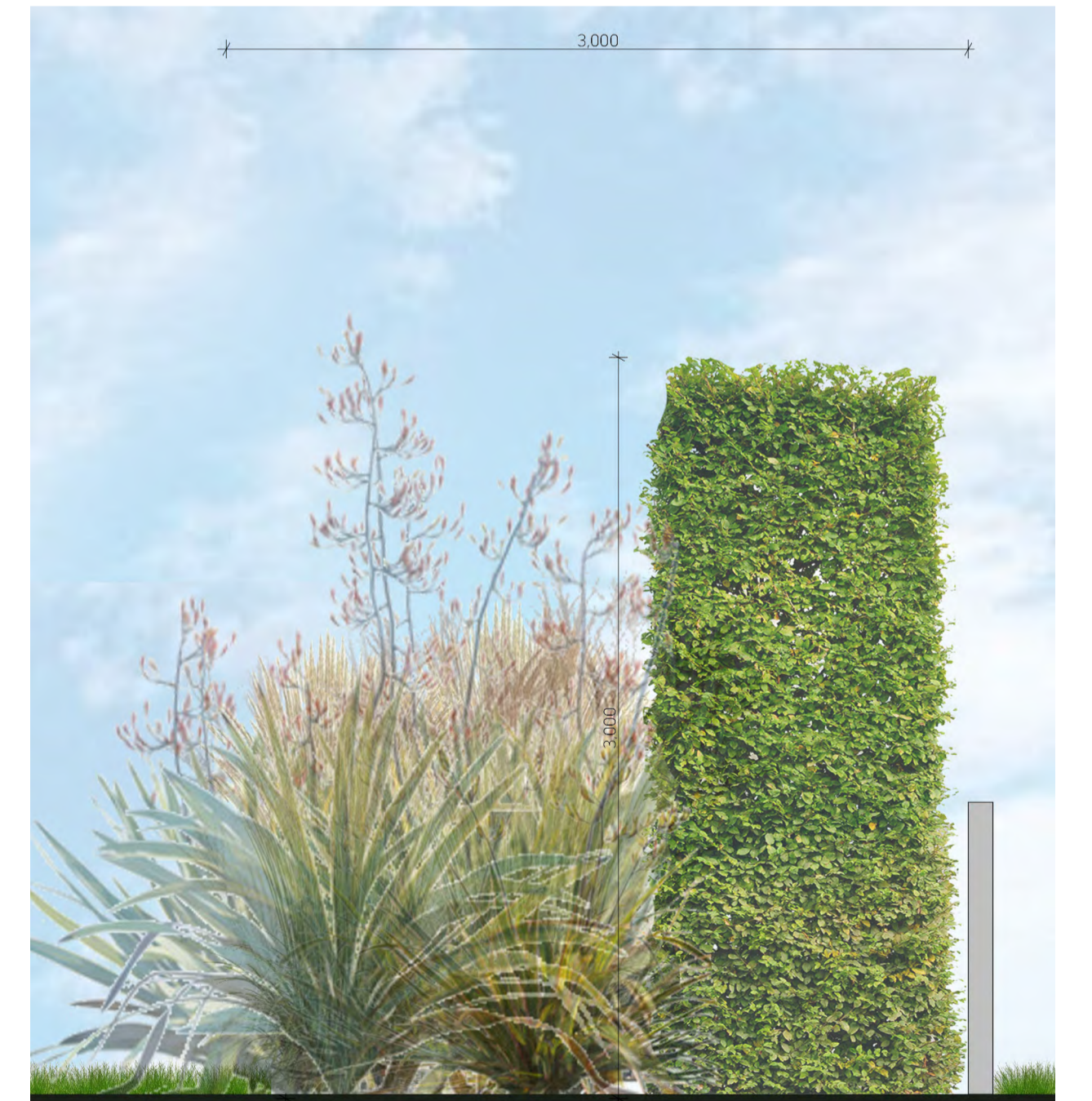
OPTION 2 - TYPICAL SECTION: 3.0m WIDE BUFFER 1:25@A1 / 1:50@A3 Note: Planting shown at 10-year maturity (expected maturity to be achieved at 5 - 7 years)
