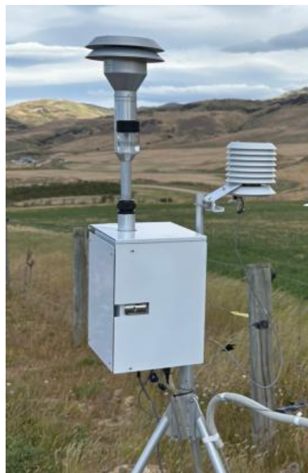
Figure 8: Photograph of real time dust monitoring equipment
