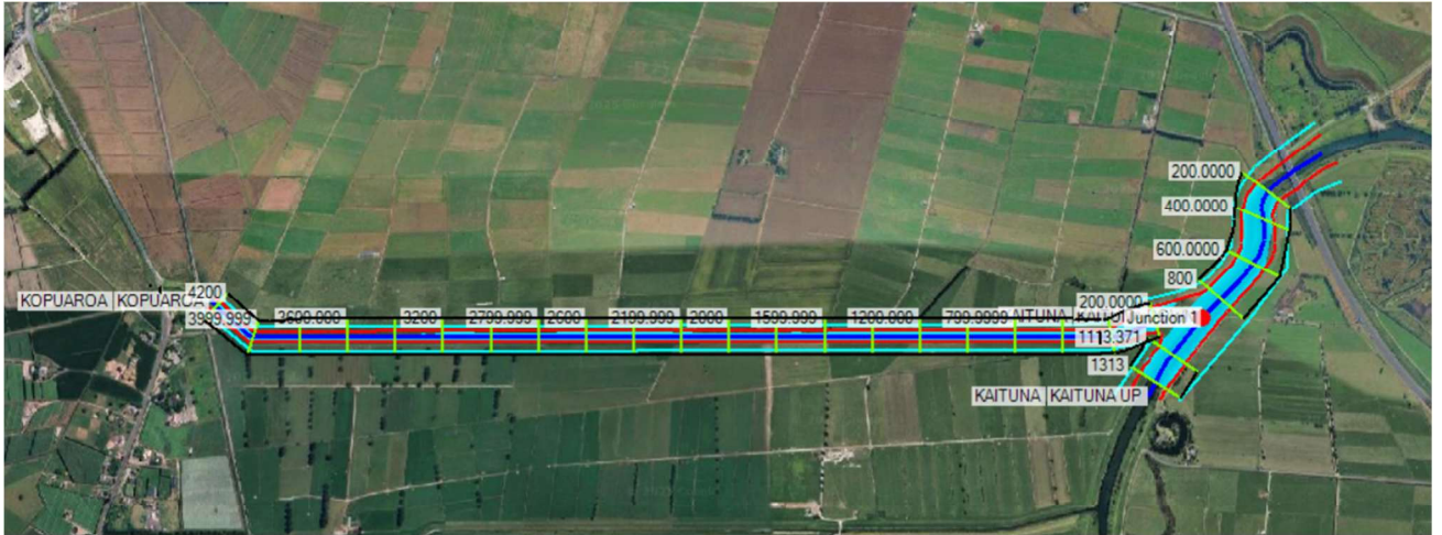
Figure 23 – Kopuaroa and Kaituna Calibration 1D (Source: HEC-RAS)
