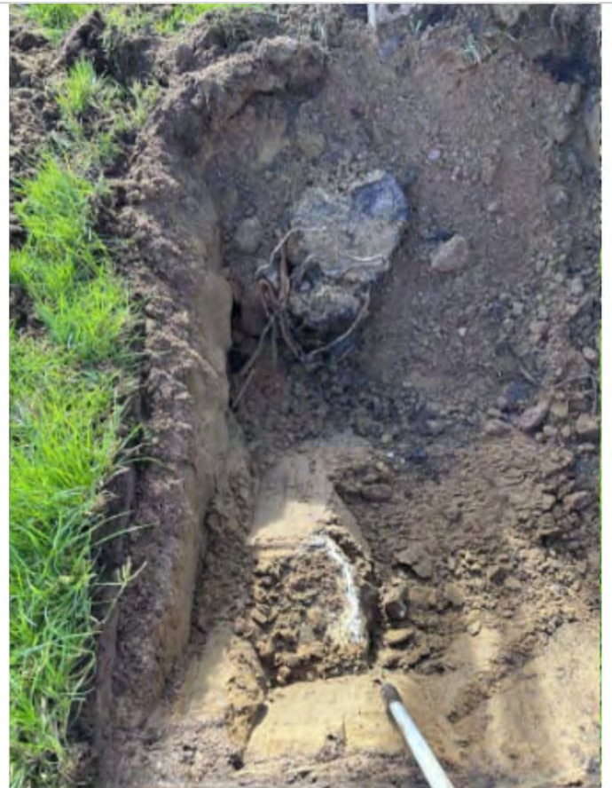
Photo 4: Waste observed in western wall of test pit adjacent to dairy shed (O5)
