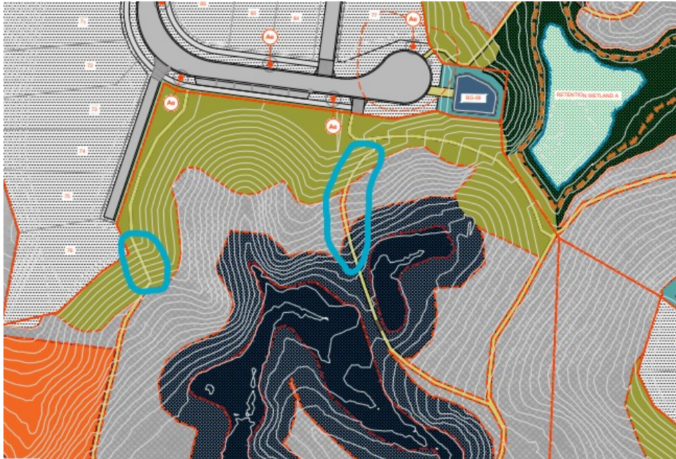
Figure 9: Example of poor track locations
