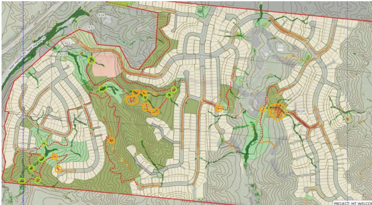
Figure 13: Overlay of proposed tracks and overland flowpaths
