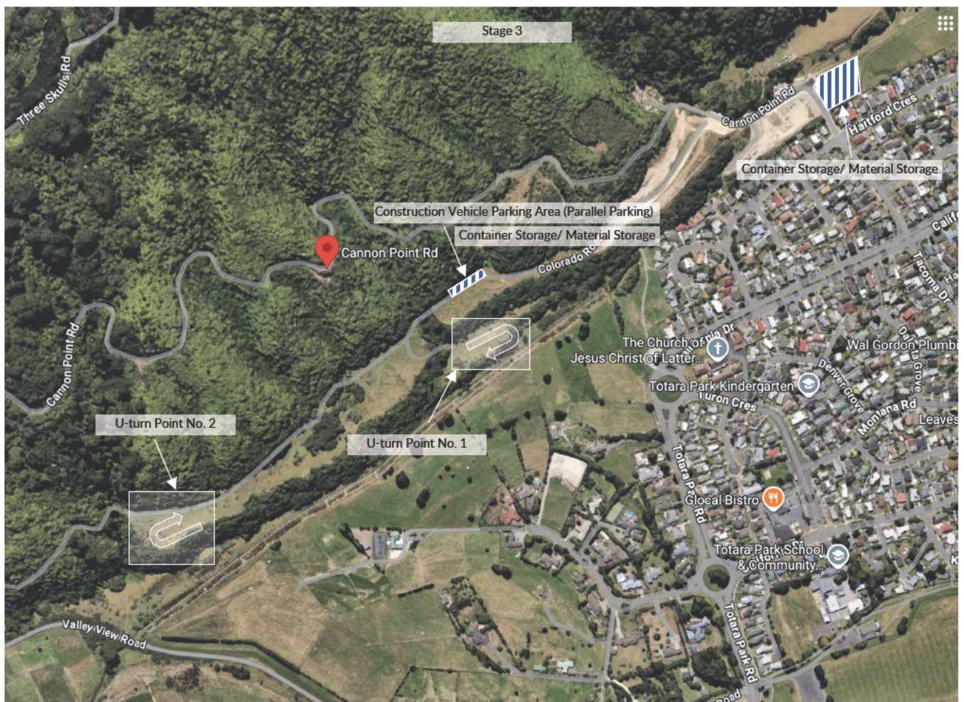
Figure 5-2 Stage 3 Temporary Construction Compound Layout
