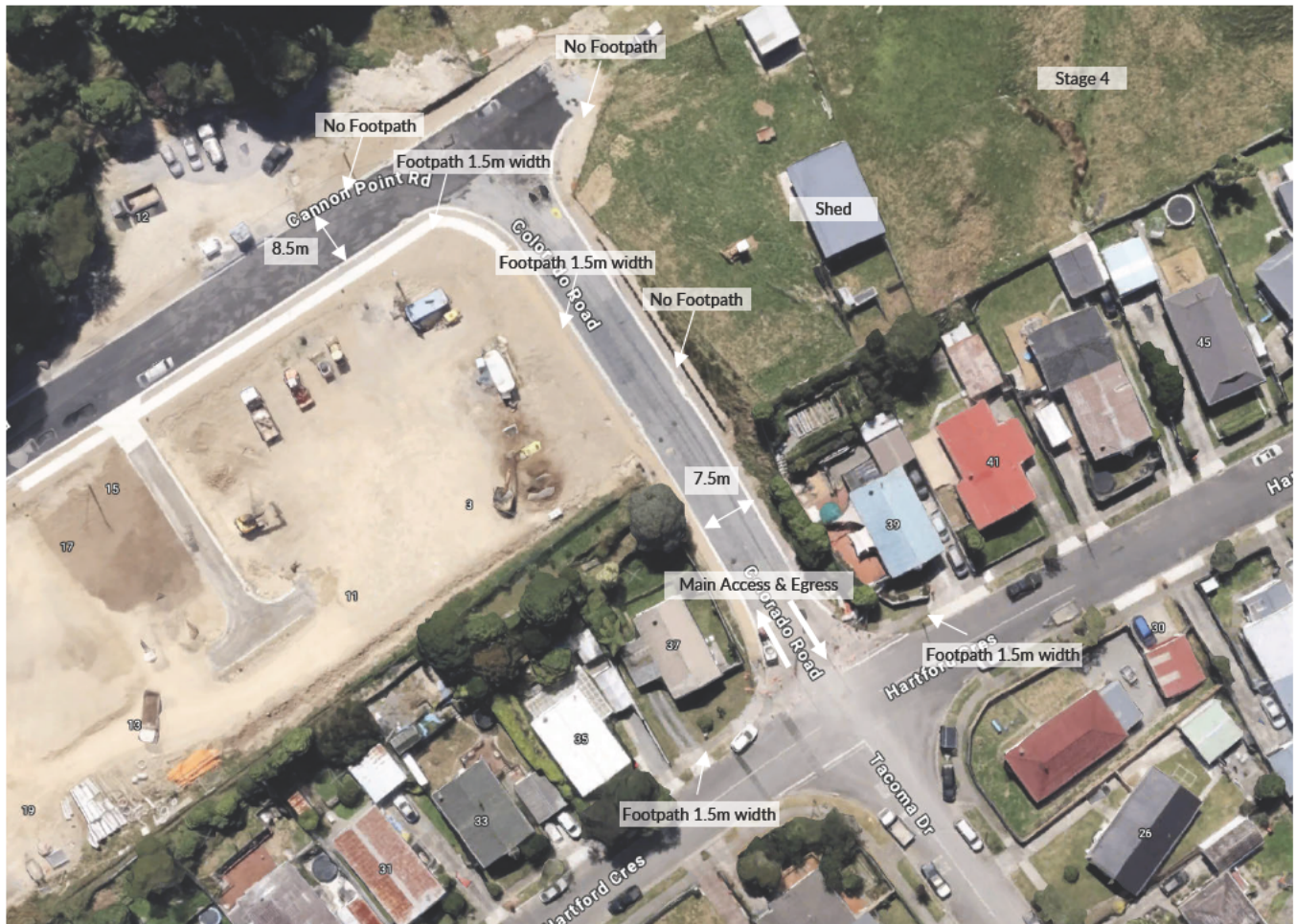
Figure 5-1 Site Access and Vehicle Routing Plan
