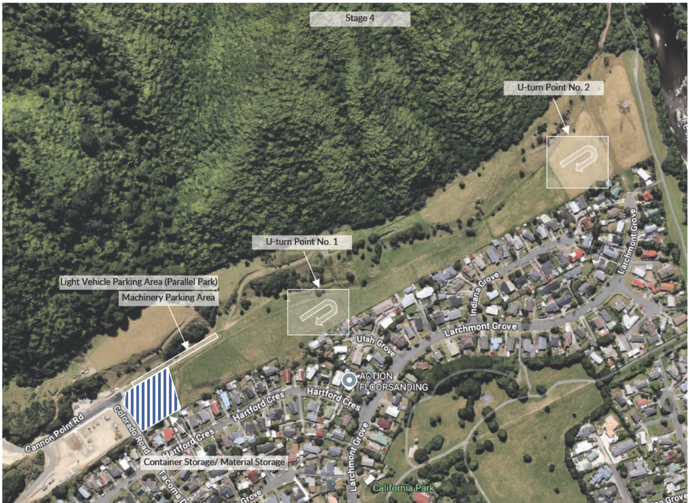
Figure 5-3 Stage 4 Temporary Construction Compound Layout
