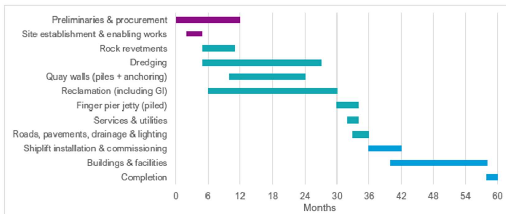
Figure 15: Indicative Construction Programme Gantt Chart (Source: Beca (2026))
