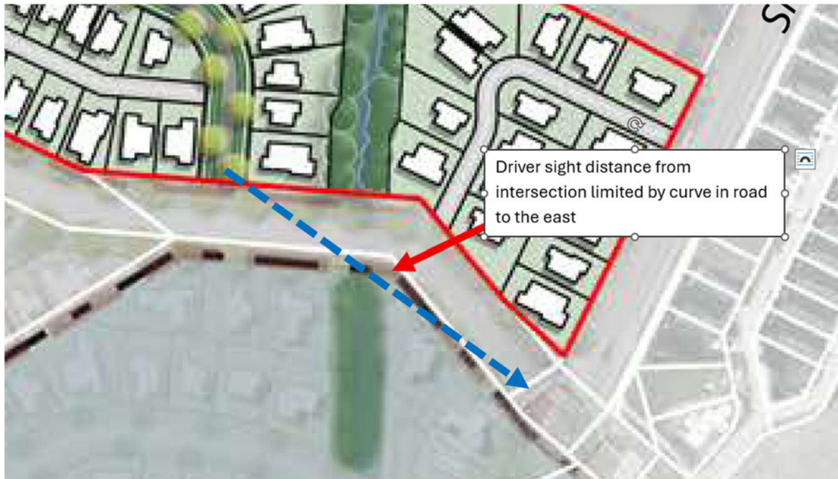
Figure 8: Example of driver sight distance from intersection limited by curve.
