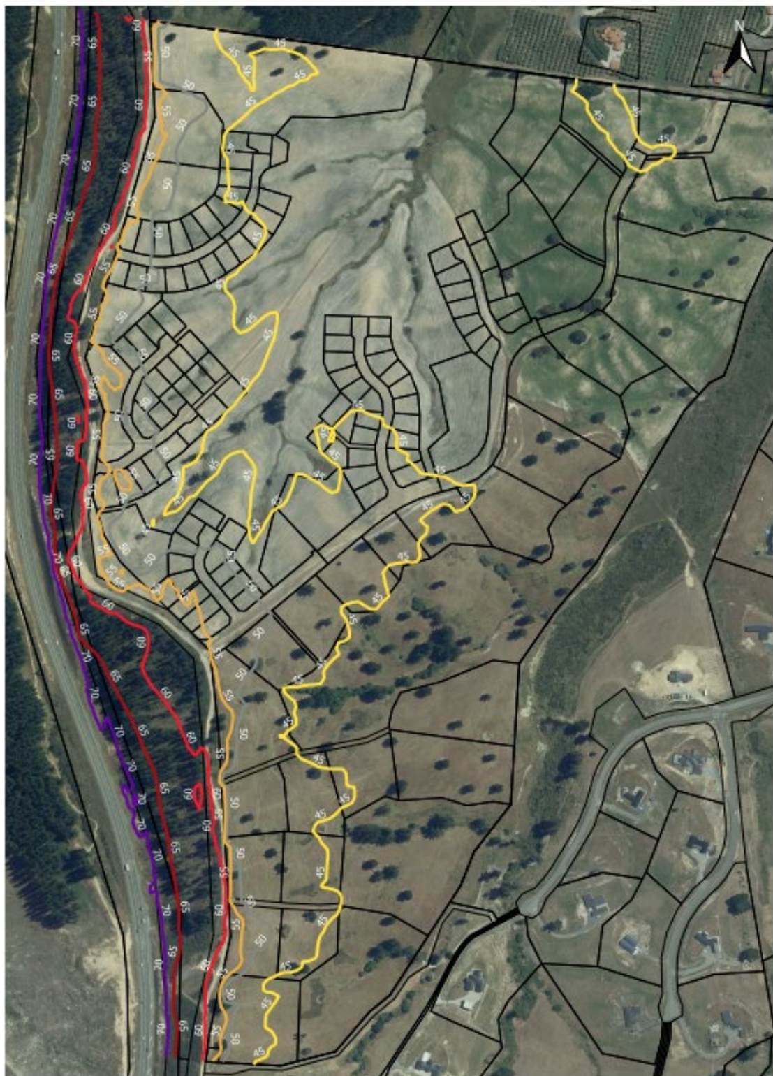
Predicted traffic noise levels at 1.5m height (ground floor) - dB LAeq(24hr) (includes +3dBA to account for future growth)
