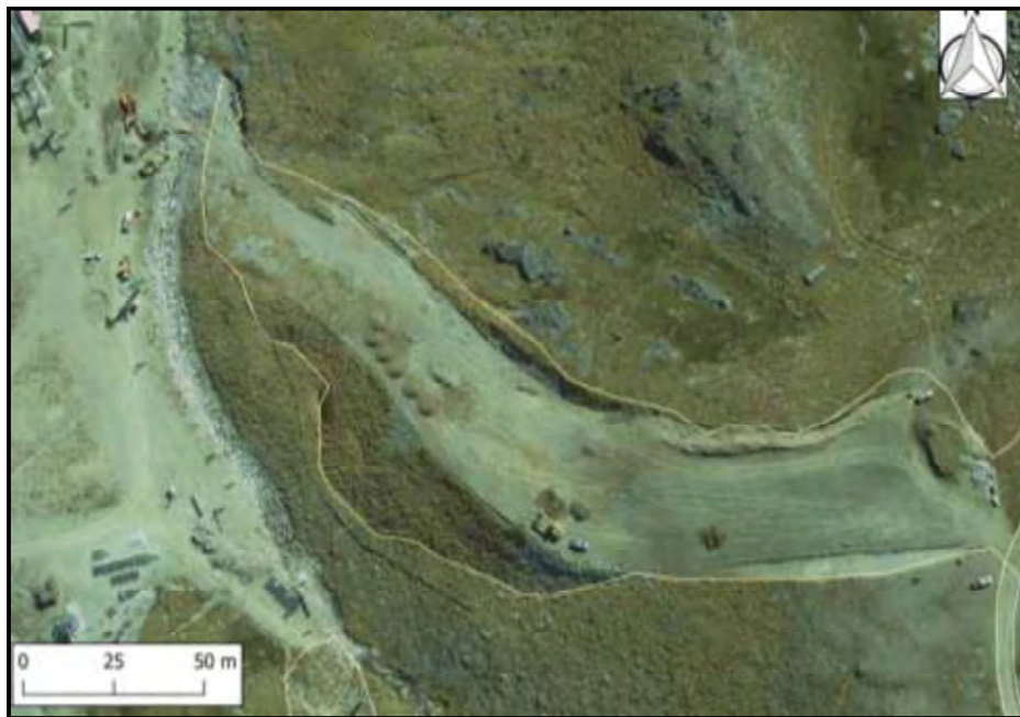
Figure 74. Aerial view of the recent work (refer Figure 71 above) with reworked area outlined in yellow and replanted area the slope below the skin trail. Note piles of saved top soil and replanted tussocks on the trail.
