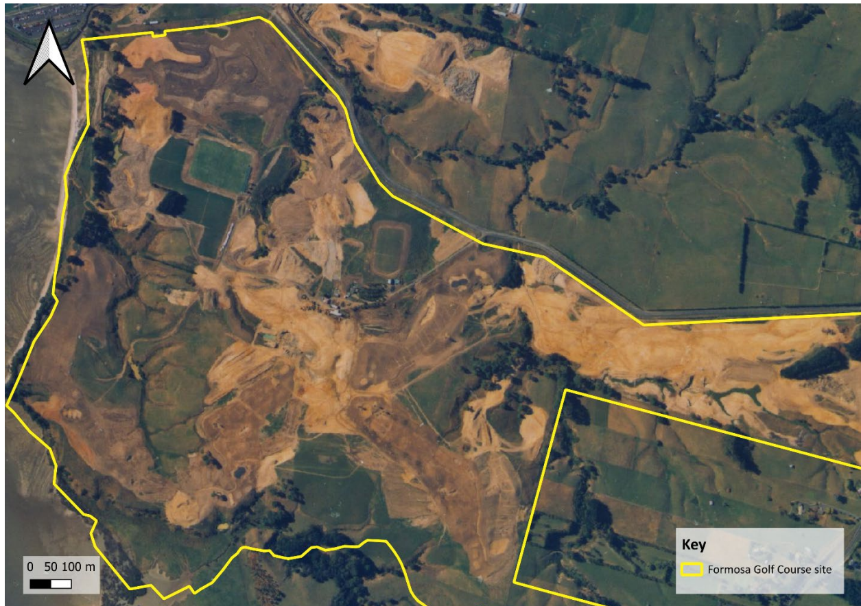
Figure 13. Historical aerial imagery from 1996 showing extensive earthworks and construction of the Formosa Golf Resort, including creation of artificial ponds, drainage features and modified landforms.
