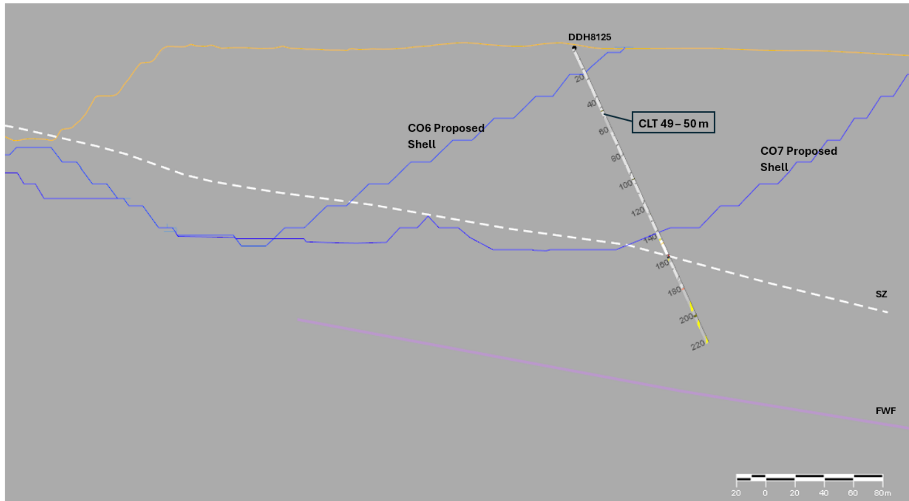
Figure A3: DDH8125 (Column 3) cross-section with CLT interval indicated.
