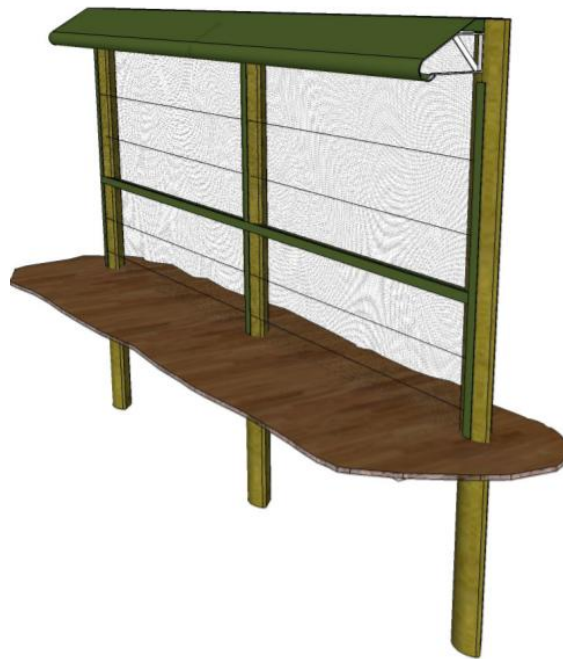
Figure 10. Diagram of a standard predator-proof fence (above and below ground),
