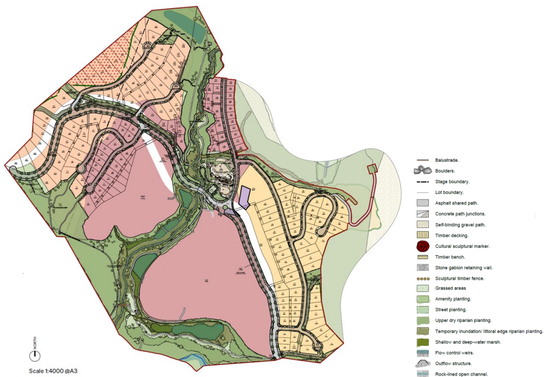
Figure 2: Proposed layout of the development overlying the NRMP zones
