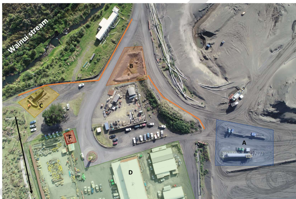
Figure 2. Stormwater management. A) Diesel fuel tank. B) Catchment area for diesel fuel tank. C) Hydrocarbon trap. D) Administration buildings catchment area. F) Petrol facility. Orange lines mark the bunding in place, to avoid runoff to reach the Wainui stream and direct any spills from the diesel tank to the catchment area. Black arrow indicates direction of water from the hydrocarbon trap to the process water system.
