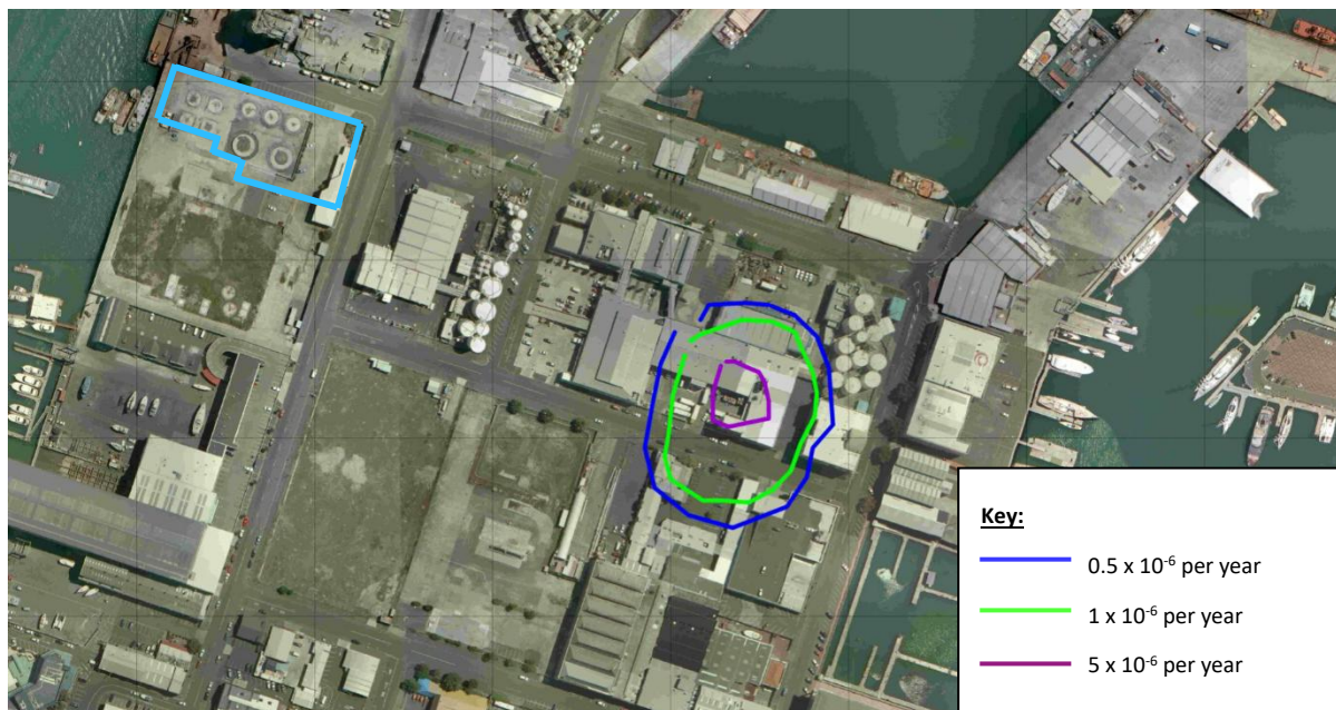
Figure 4.4: Individual fatality risk contour for the Sanford Fish Processing Plant (Figure reproduced from QRA 2011 Addendum report, doc ref 20359-QRA-009). Location of the site is indicated in light blue.
