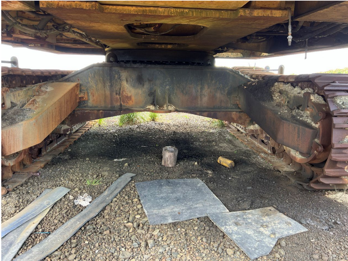
Photograph 5: Extension of the Graveyard area with weathered hydrocarbon staining under heavy machinery where PMS09 was sampled.
