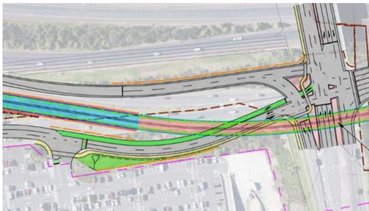
Figure 6 – Option 7, showing the realignment of Gunton Drive and the onramp to SH18.
