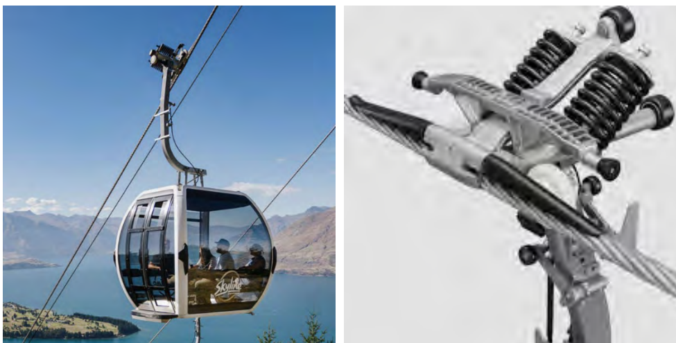
Figure 28. Detachable carrier and an example of the carrier rope grip
