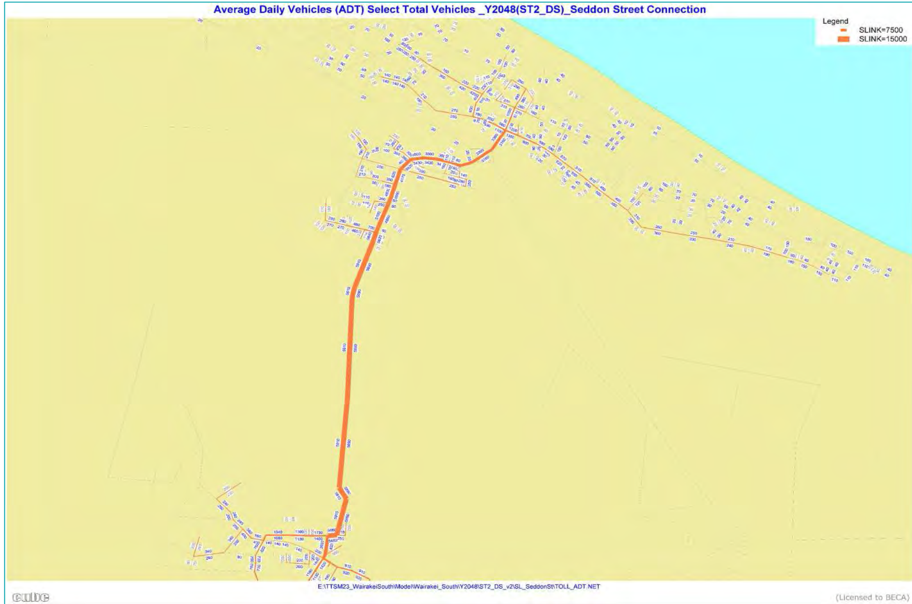
Figure 3-7: Select Link Travel Pattern for 2048 Sensitivity Test 2 land use with Do Something Network
