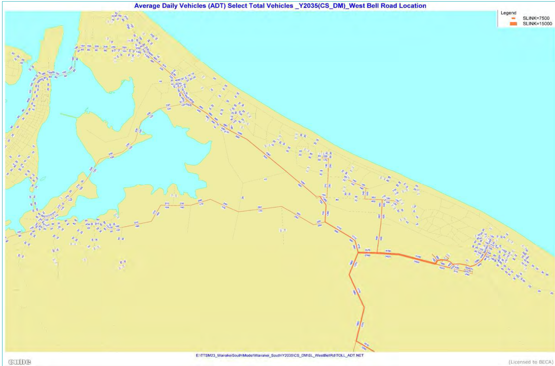
Figure 3-4: Select Link Travel Pattern for 2035 Core Scenario land use with Do Minimum Network – West Bell Road Location
