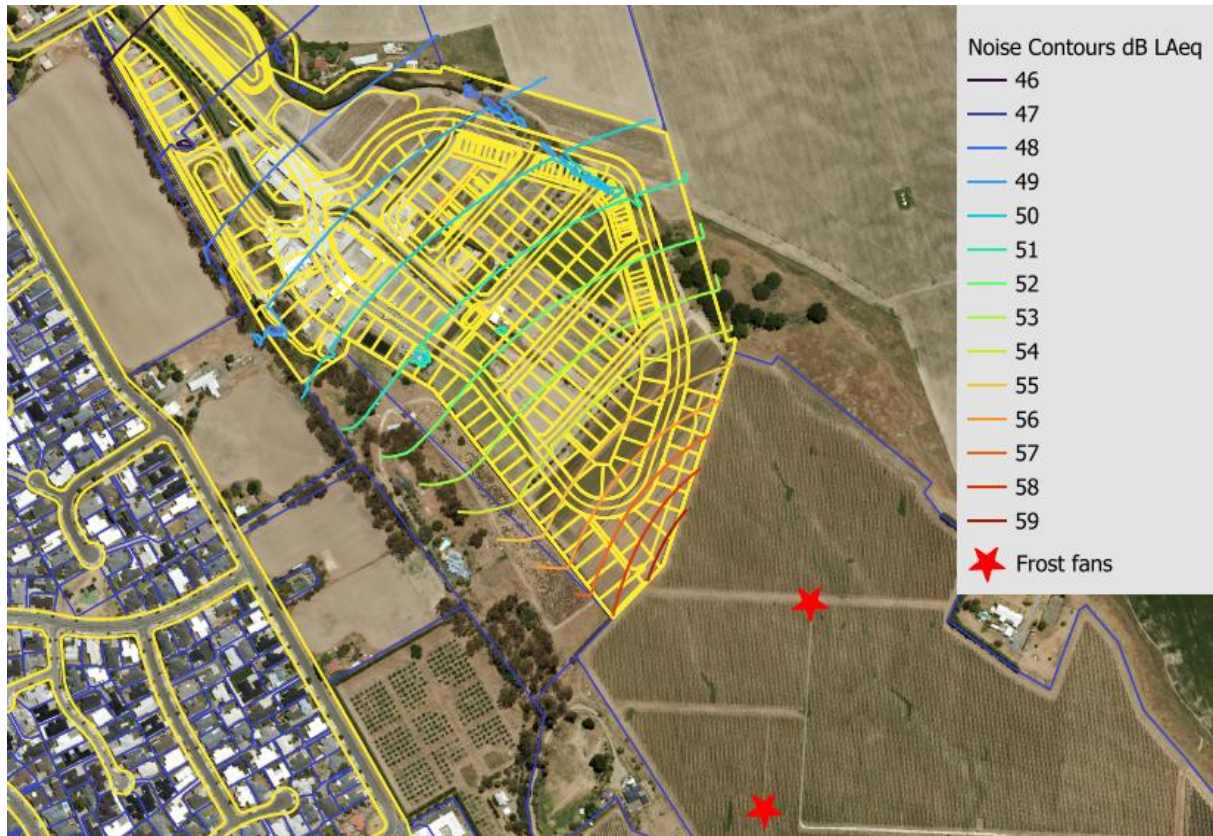
Figure 6 Cumulative noise level predictions for two frost fan machines
