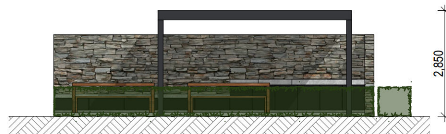
E01 PERGOLA - ELEVATION Scale 1:100
