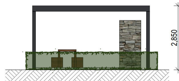
E02 PERGOLA - ELEVATION Scale 1:100
