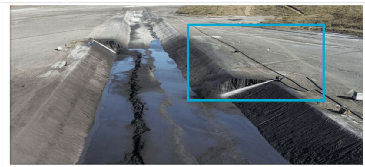
Figure 7-4 Flexible ROMU supply mining hose
