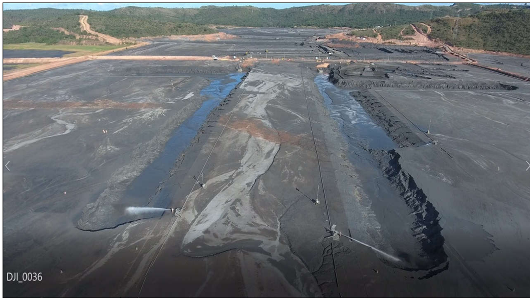
Figure 5-9 Launder development during Hydraulic Mining
