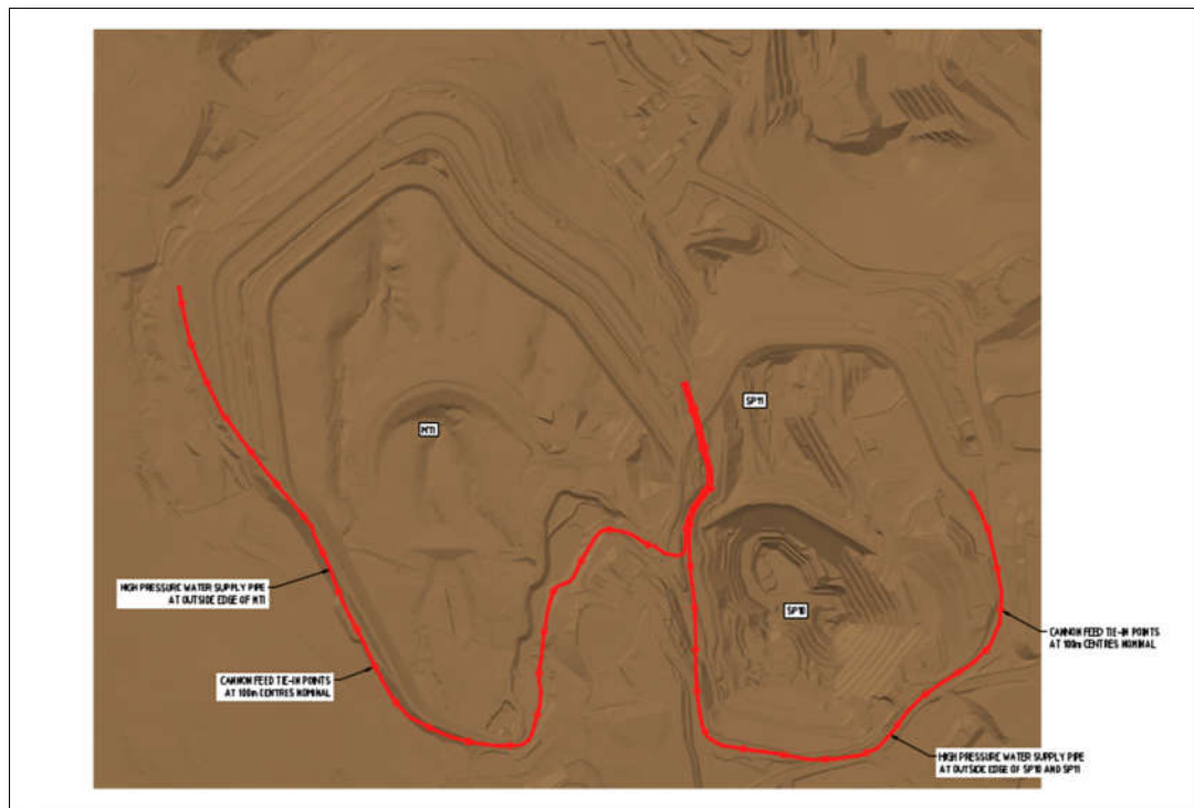
Figure 7-3 Preliminary High Pressure Supply Steel Pipeline
