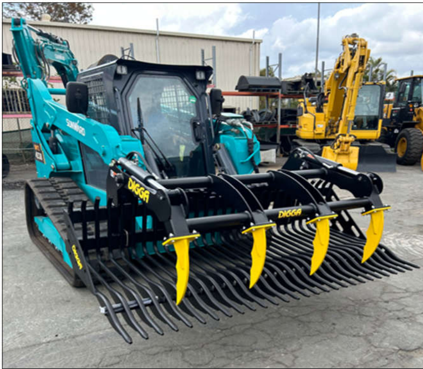
Figure 7-5 Skid Steer Loader with pipe grab attachment
