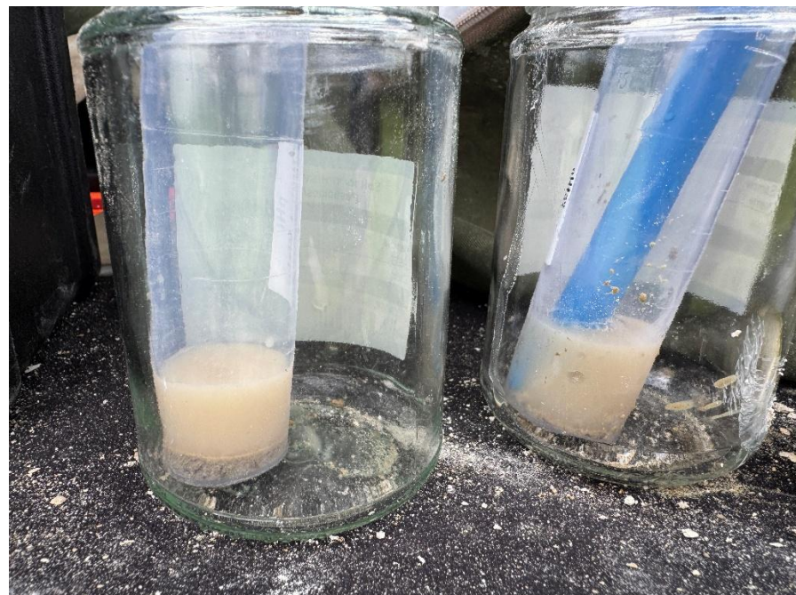
Photo 9: ASS05_1.25 m bgl – pHF (right) and pHFOX (left) reactions (17 February 2026).
