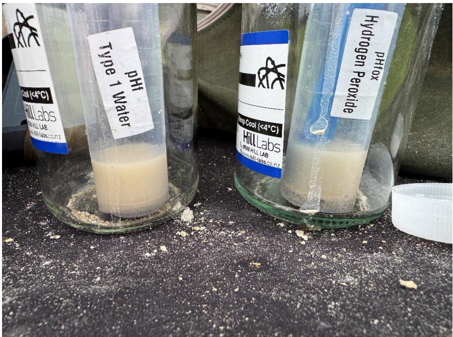
Photo 11: ASS06_1.5 m bgl – pHF (right) and pHFOX (left) reactions (17 February 2026).
