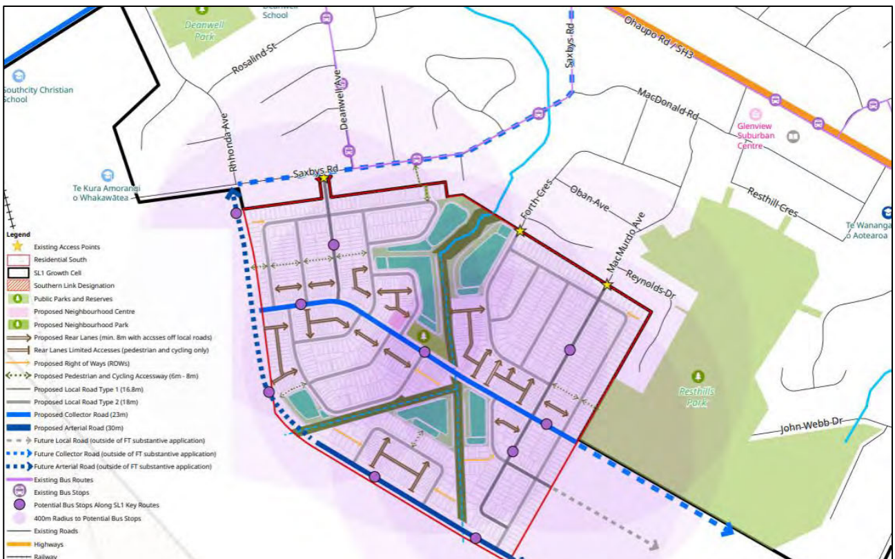
Figure 36: Residential Development – Road Carriageway Width Hierarchy
