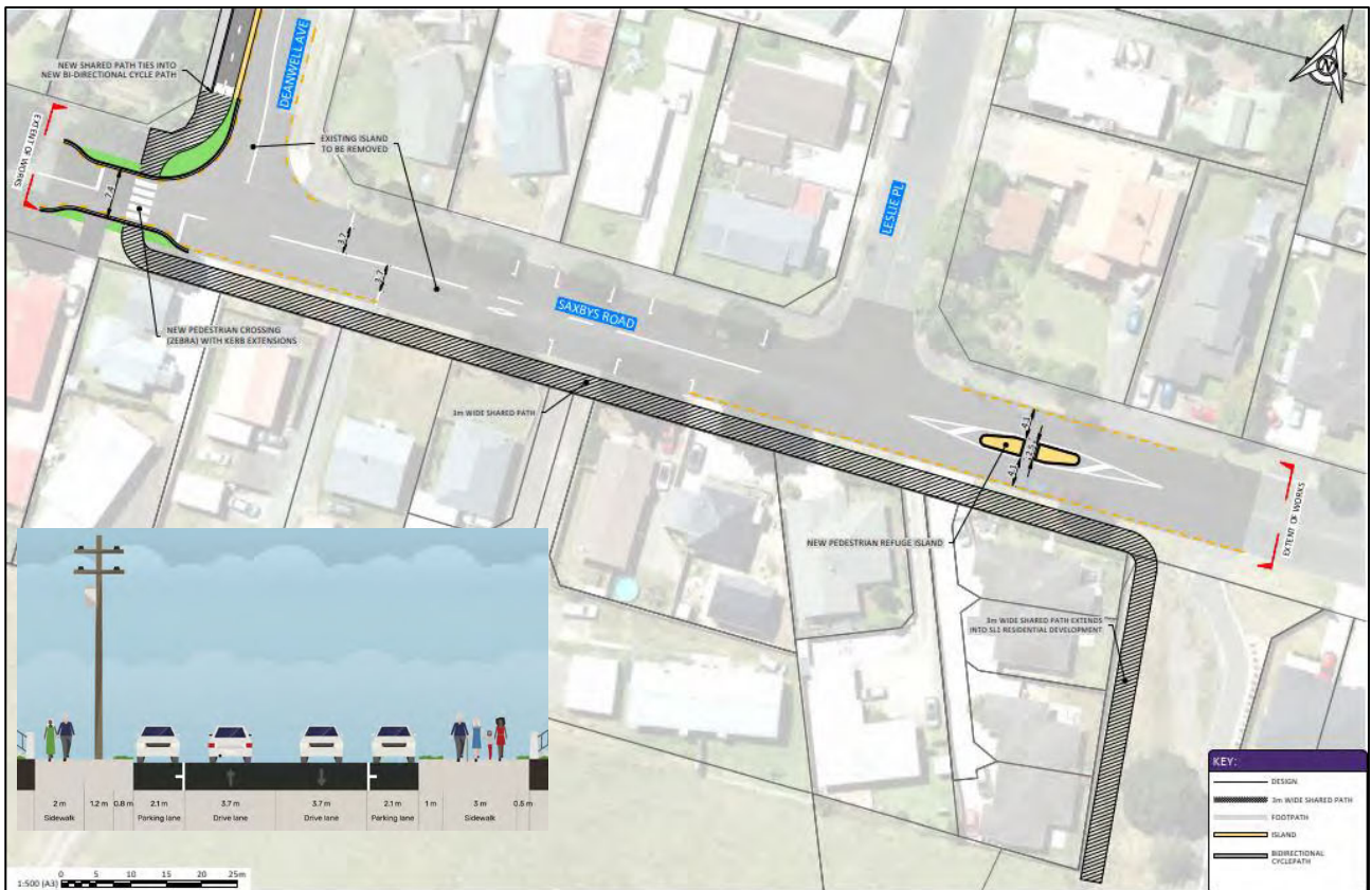
Figure 28: Indicative Alignment and Cross-section of Saxbys Rd
