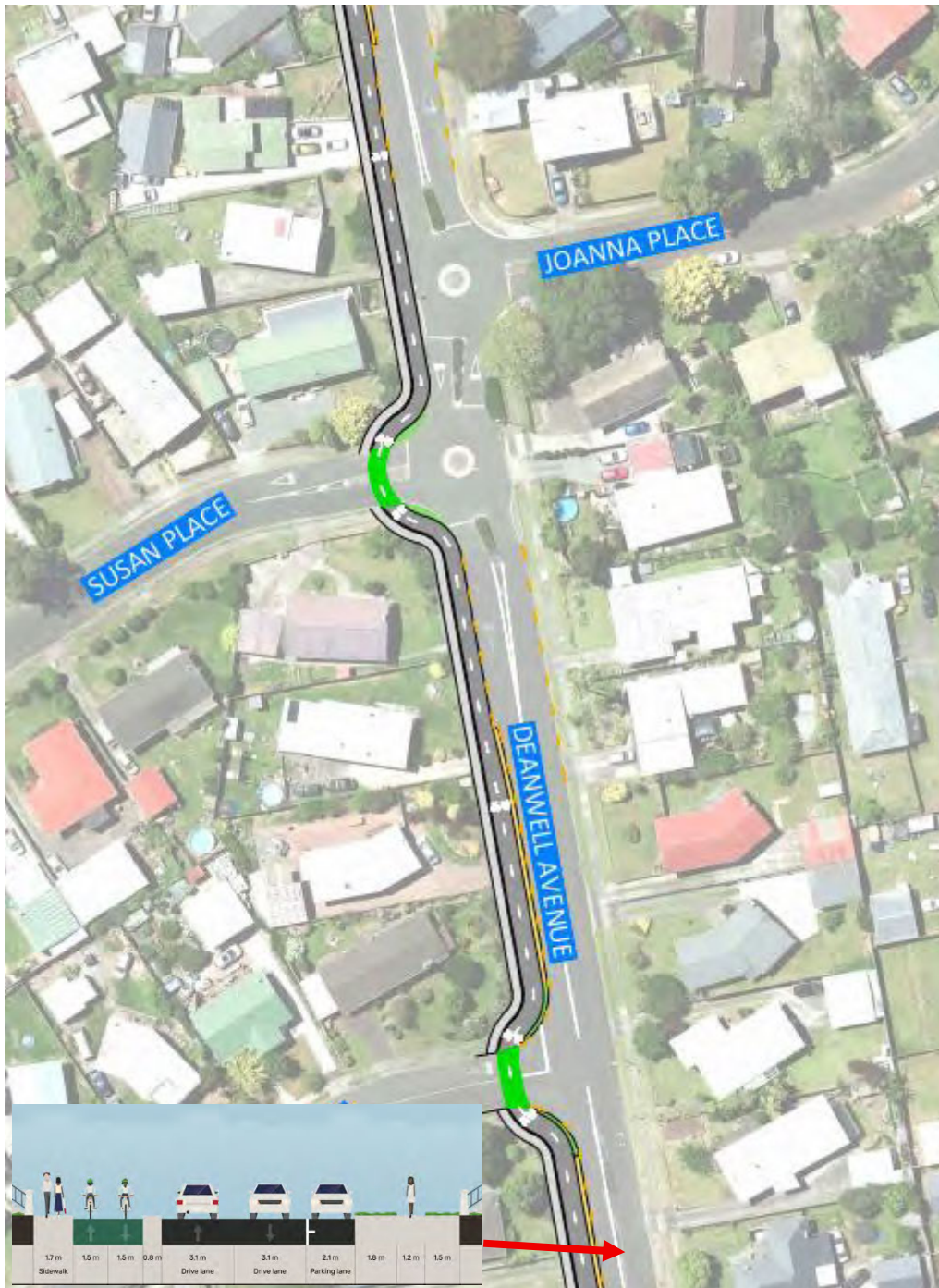
Figure 31: Indicative Alignment and Cross-section of Deanwell Ave
