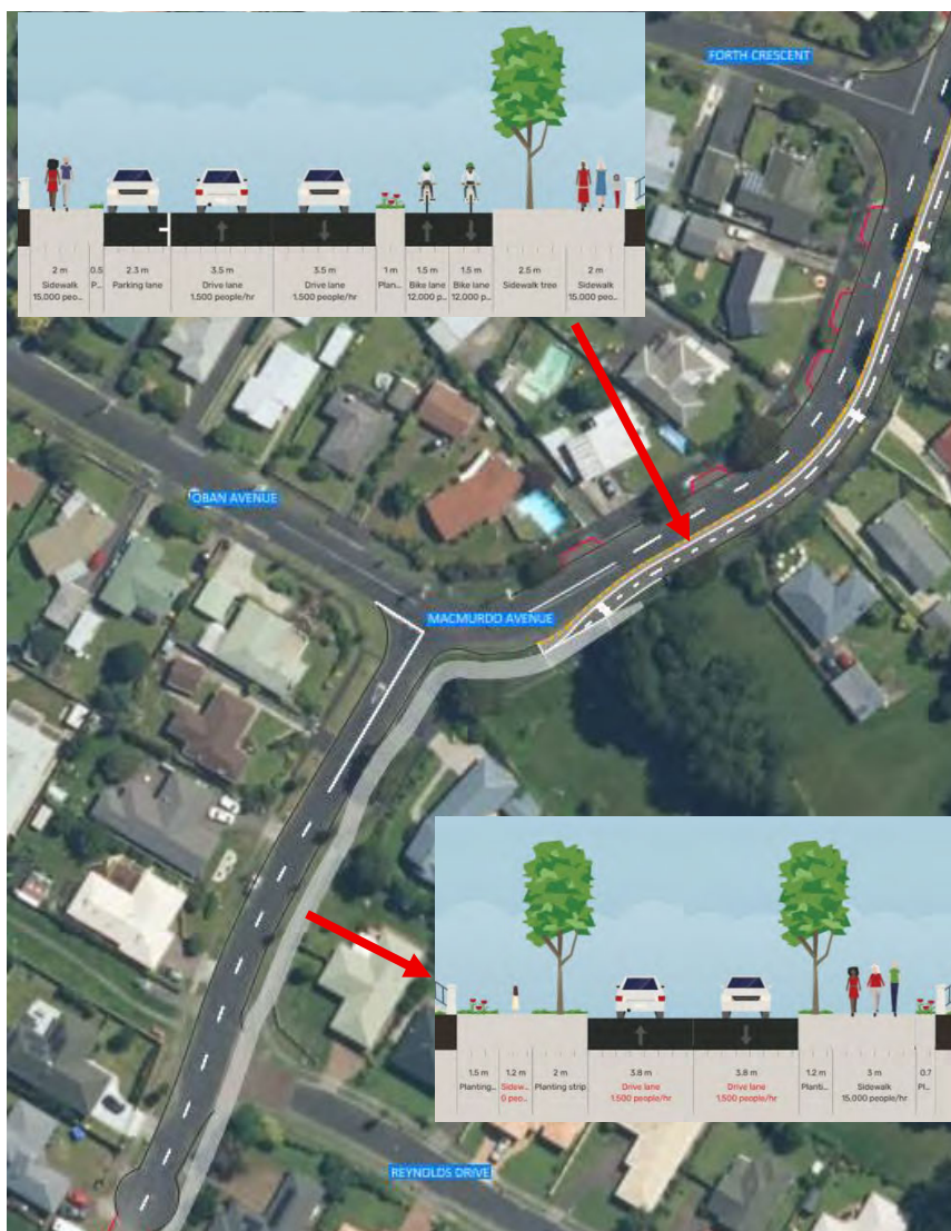
Figure 30: Indicative Alignment and Cross-section of MacMurdo Ave
