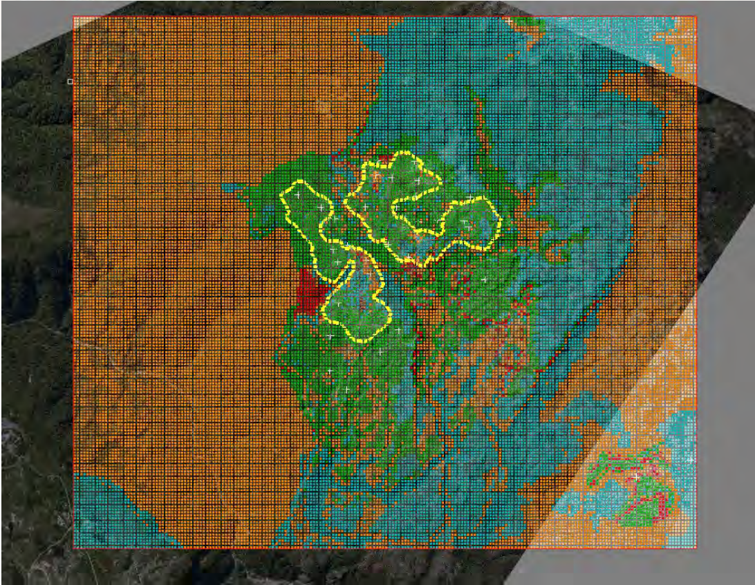
Figure 14. The MFS ABA Model coloured by the MFS PFC (only surface blocks shown: 0.5 m – 2.0 m below surface). Green = NAF, Cyan=Low Risk, Orange = PAF, Red = HAF. MFS Pit Shell design shown (dashed yellow).
