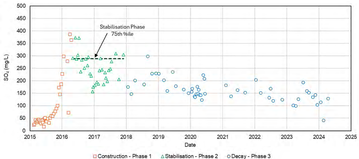
Figure 41. Derivation of SOX load from BV ELF sulfate data.
