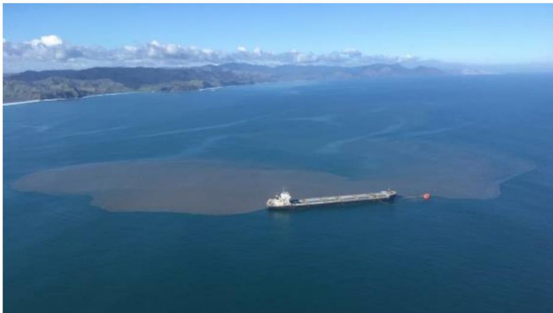
Figure 1.3 Plume of water and fine particles discharged during ship loading operation. Source: personal communication with Jared Pettersson (Enviser).
