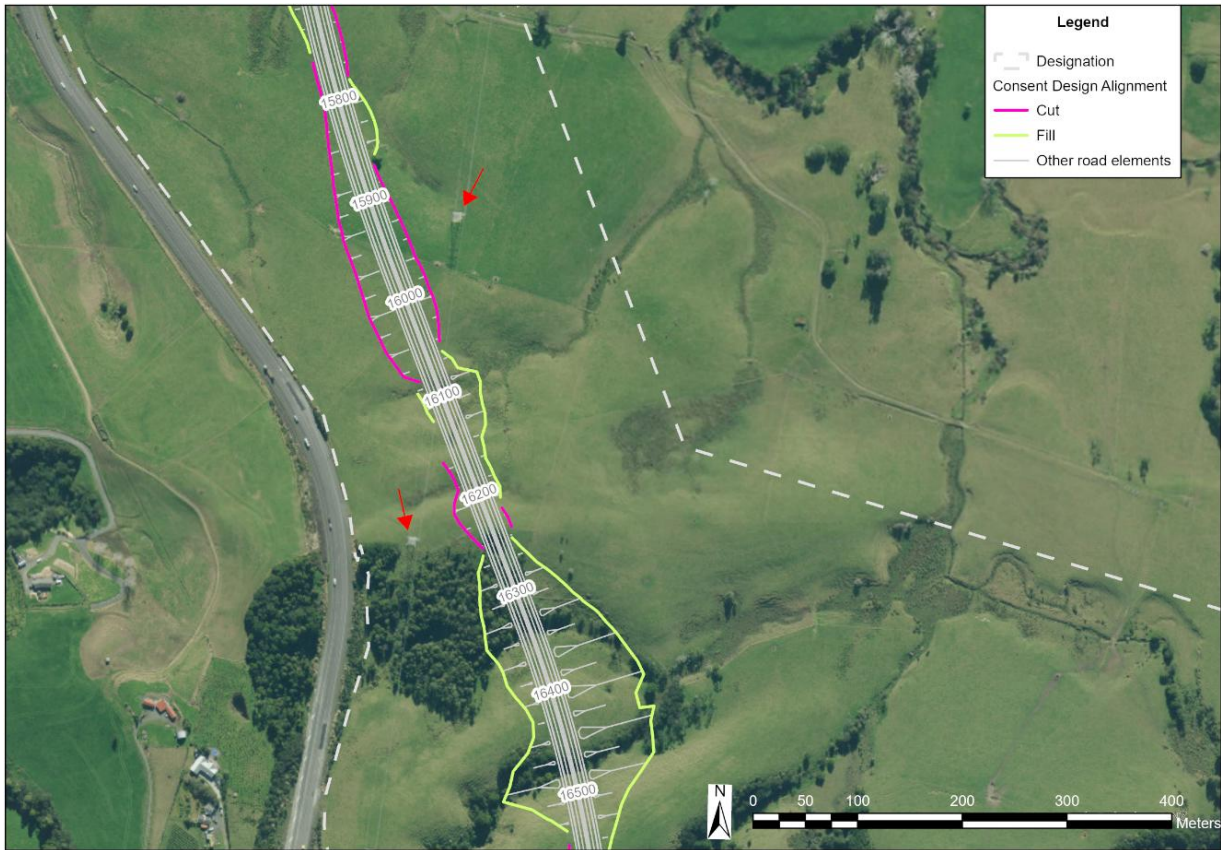
Figure 13: GIS map showing location of Transpower pylons relevant to proposed cuts in Waipapa profile (the closest pylons next to the cuts)
