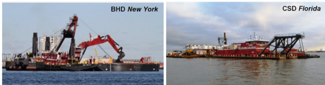
Figure 12: Photographs of each of the dredging plant used to represent the possible dredging equipment for the project.
