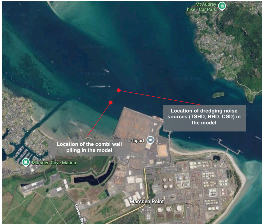
Figure 15: Source locations for the percussive piling and dredging for the acoustic model.
