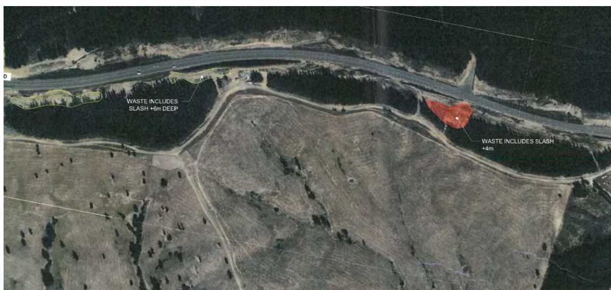
Figure 4 – Excerpt from letter to TDC “Waste Spoil Dump Sites from the construction of The Ruby Bay Bypass (February 2013)”
