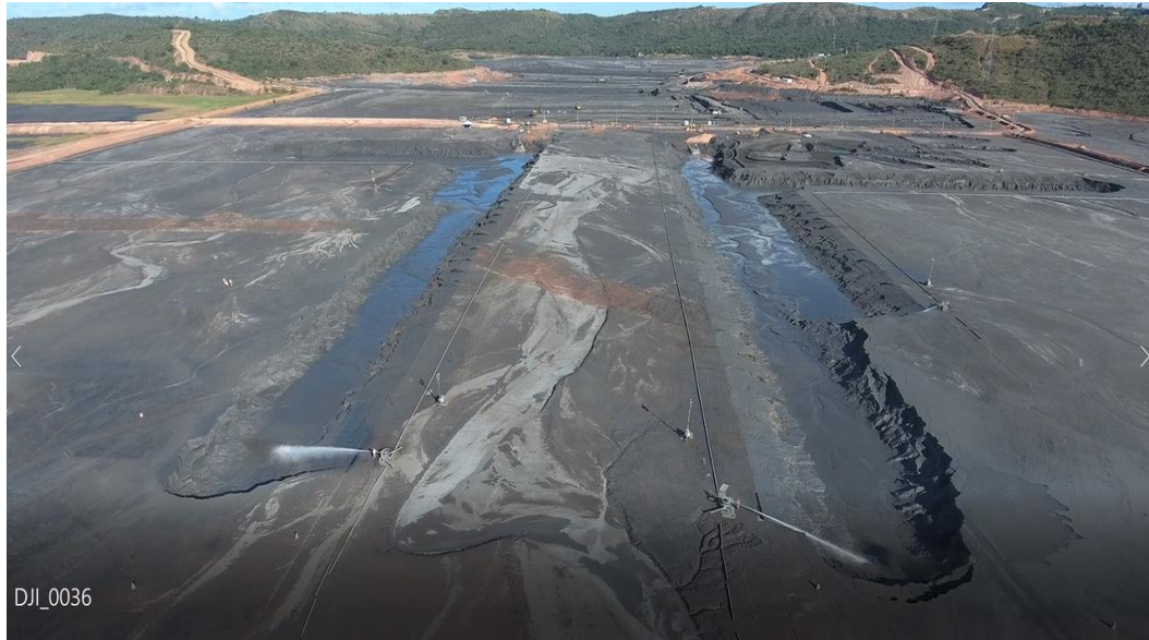
Figure 12: Launder Development during Hydraulic Mining
