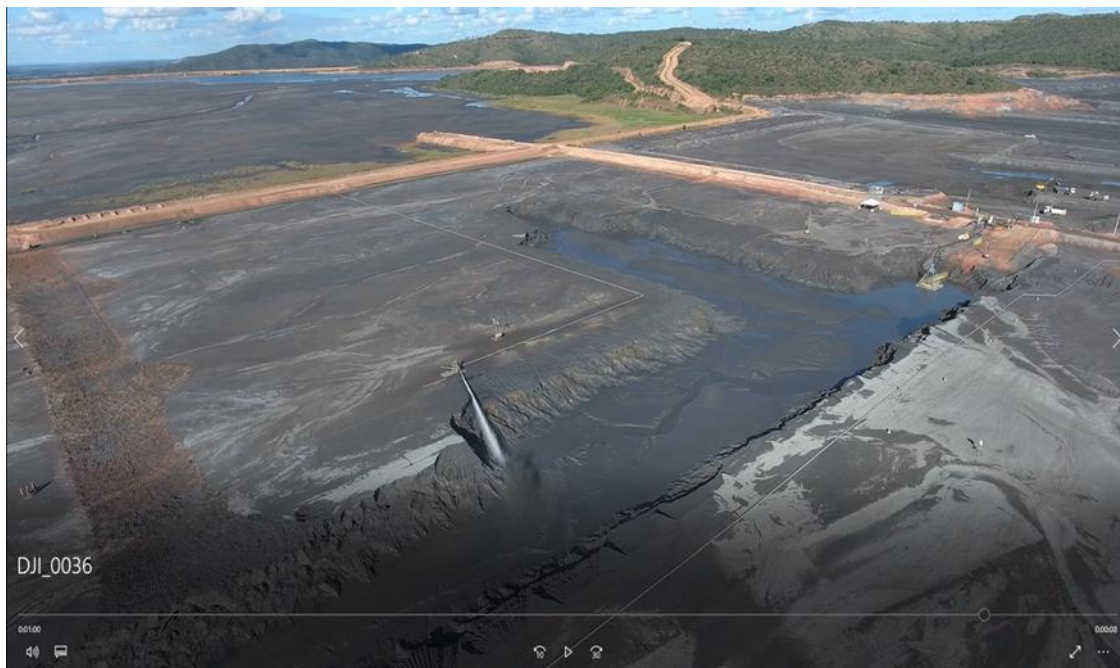
Figure 14: Bench and Mining Block Development during Hydraulic Mining
