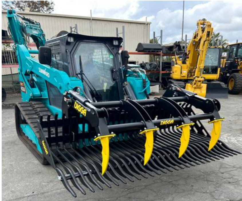
Figure 27: Skid Steer Loader with Pipe Grab Attachment
