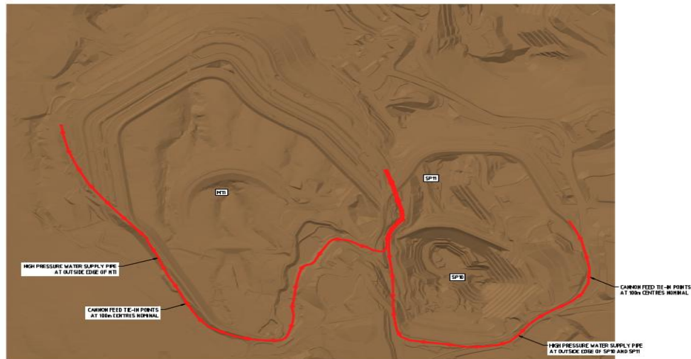
Figure 4: Preliminary High Pressure Supply Steel Pipeline
