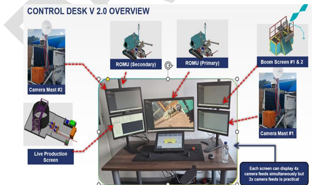
Figure 5: Remote Mining Unit Command Centre
