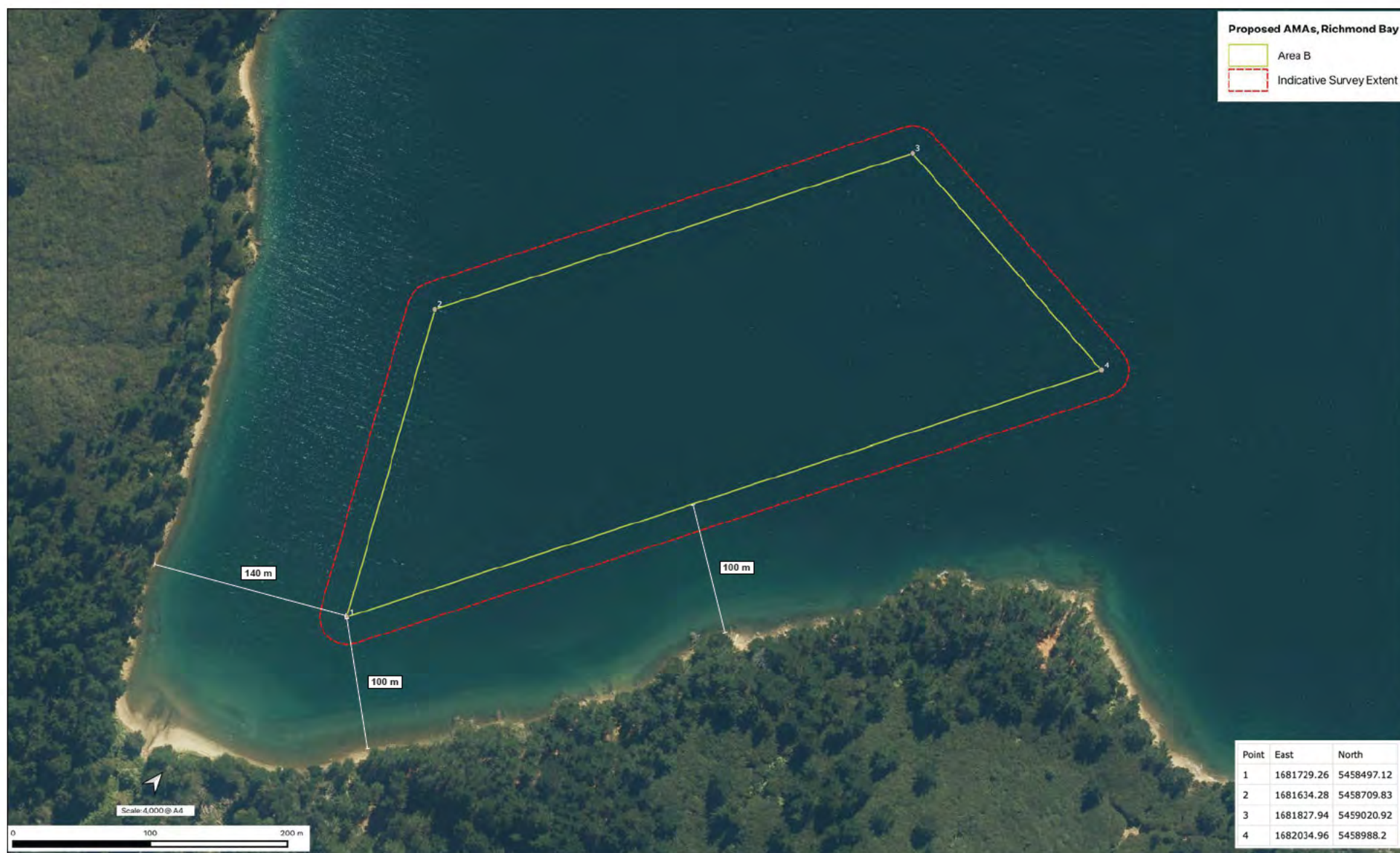
Figure H-1B Overview of Area B, surveyed area, and boundary corner locations for the proposed farm. Distances between Mean Low Water and the inshore farm boundary also shown.
