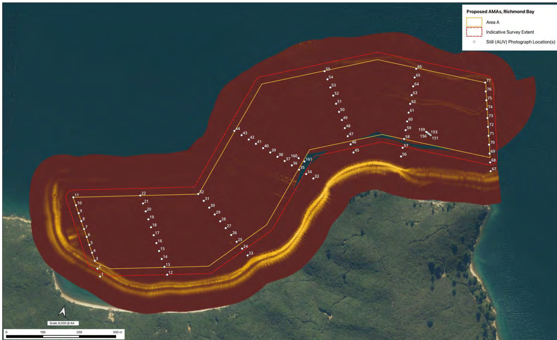
Figure H-2A Area A - Side-scan sonar image overlaid with AUV video transect and still photograph locations used to ground-truth benthic habitat features identified in the sonar data.
