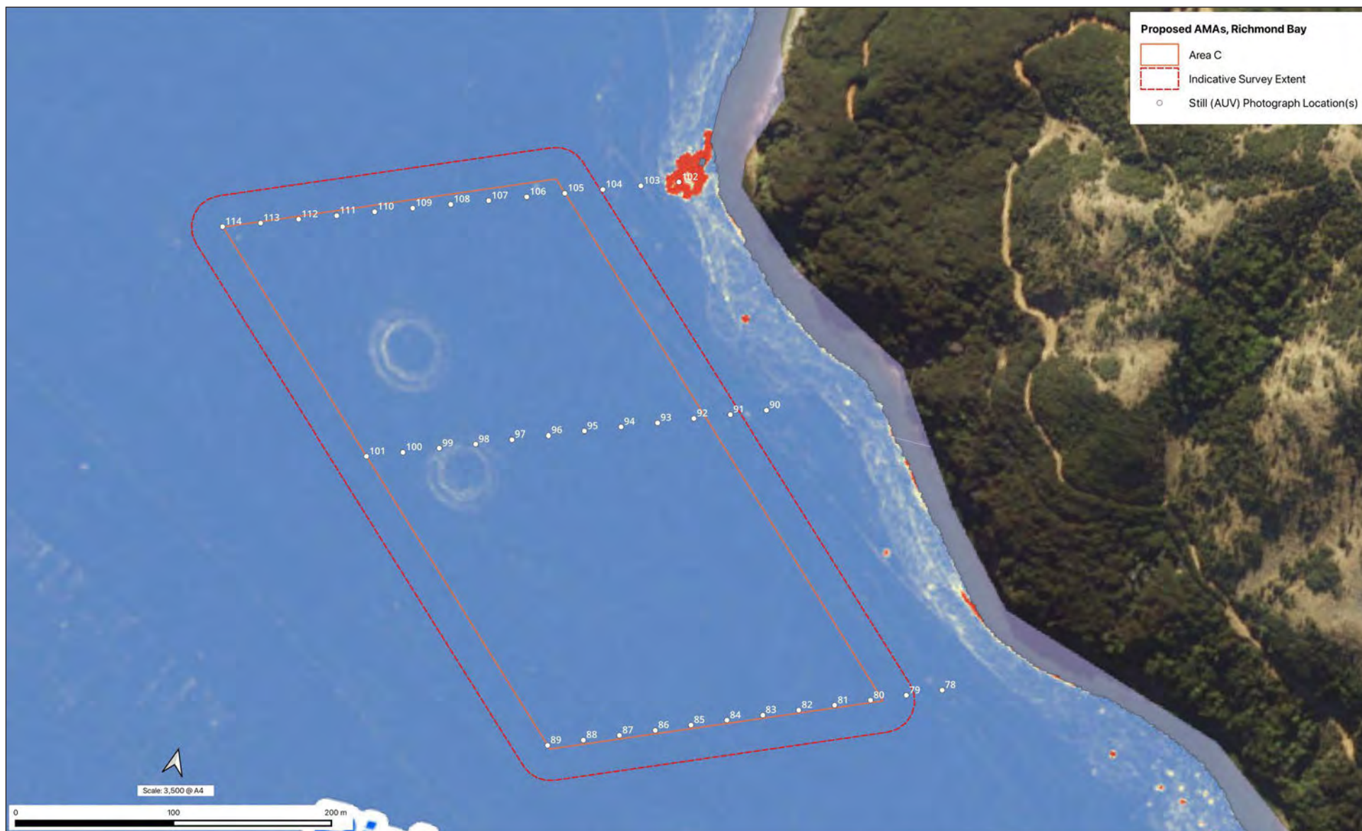
Figure H-3C Area C - MDC MBES Rugosity image overlaid with AUV video transect and still photograph locations used to ground-truth benthic habitat features identified in the sonar data.
