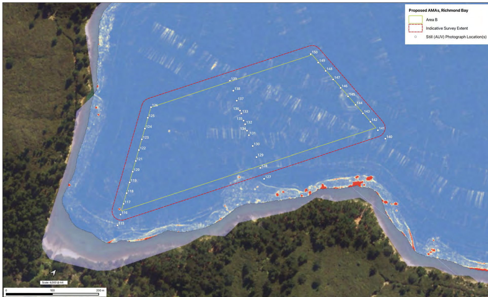
Figure H-2B Area B - MDC MBES Rugosity image overlaid with AUV video transect and still photograph locations used to ground-truth benthic habitat features identified in the sonar data.
