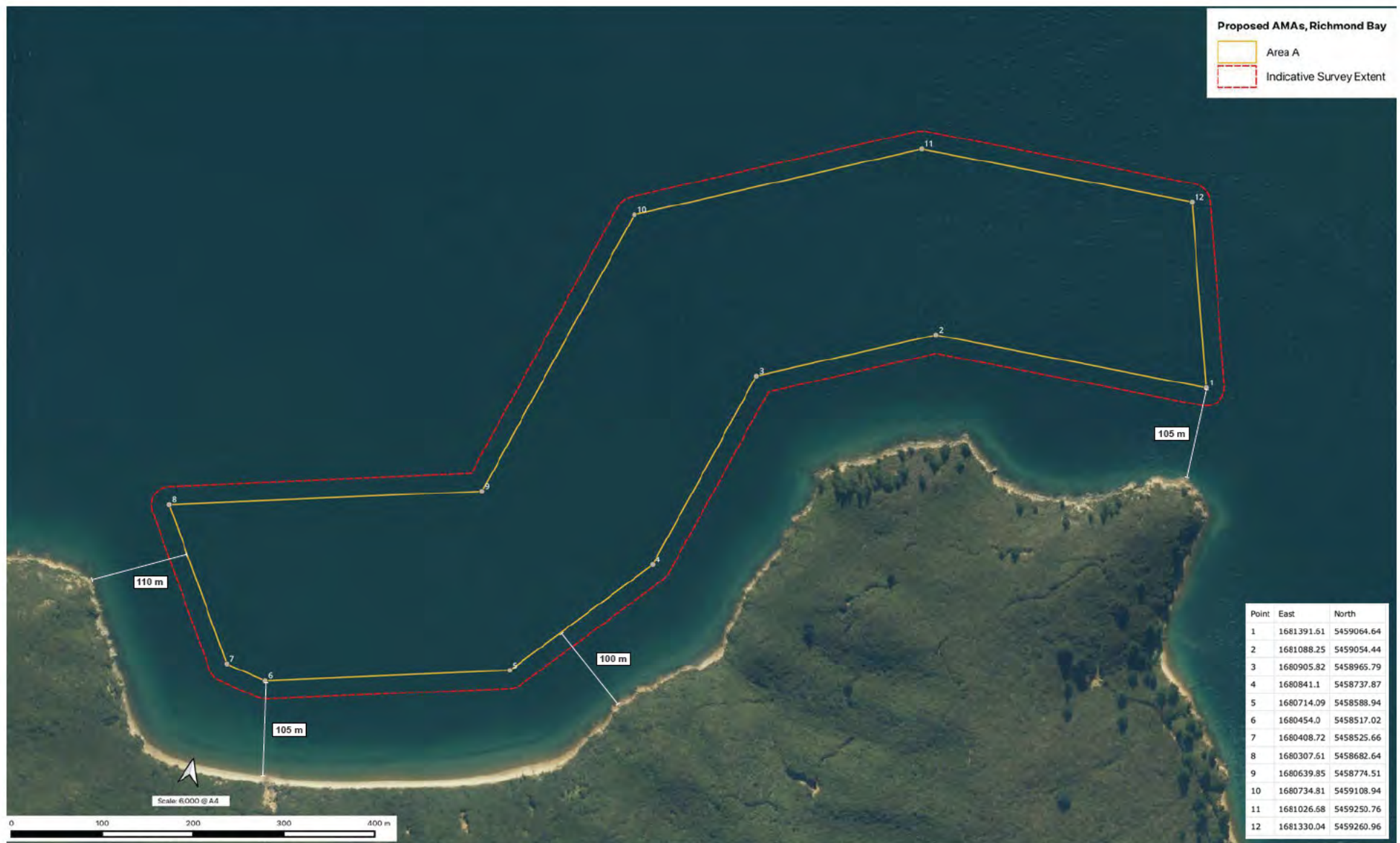
Figure H-1A Overview of Area A, surveyed area, and boundary corner locations for the proposed farm. Distances between Mean Low Water and the inshore farm boundary also shown.
