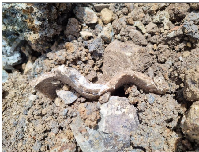
Photo 1: Fibre cement fragment ('Super-6' roofing tile)
