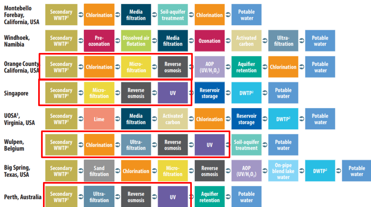
Figure 2.1 Examples of potable reuse schemes
