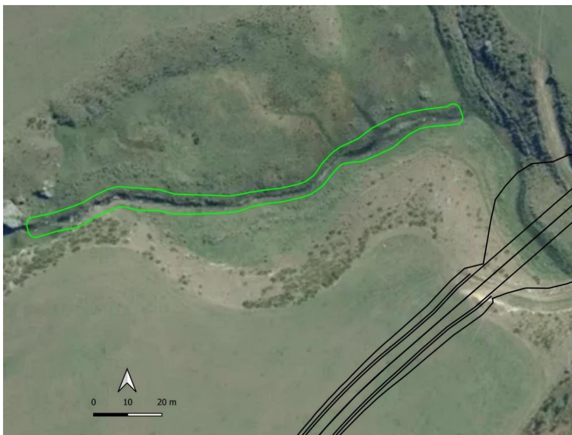
Figure 7. Diagram from SLR Aquatic Ecology Report 38 indicating proposed section of stream to be rehabilitated upstream of the proposed culvert.
