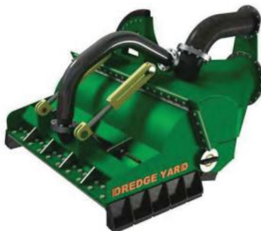
Figure 58: Typical active TSHD Drag-Head (Source: Dredge Yard).
