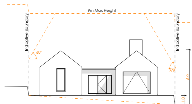
Street Elevation cross fall site
