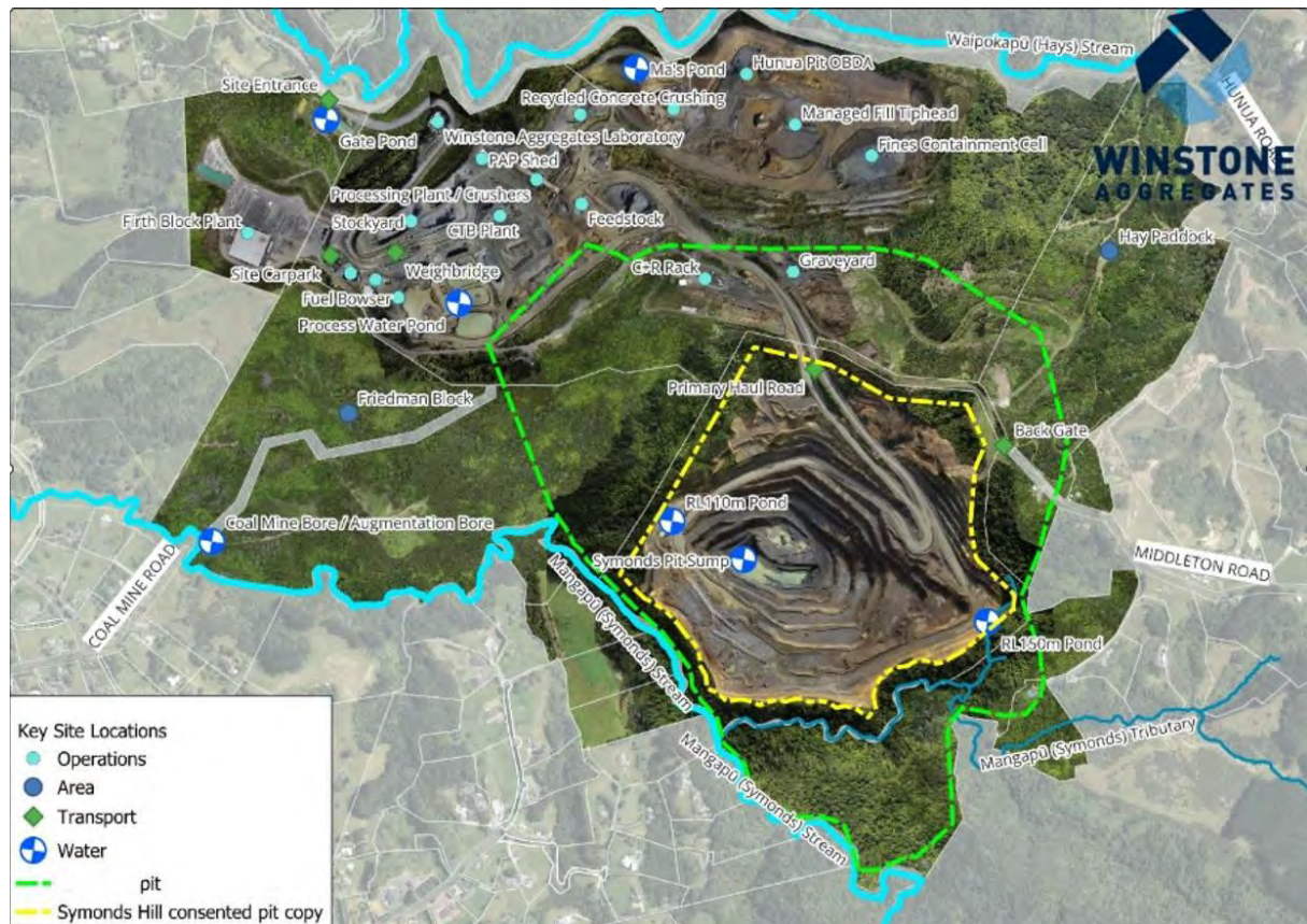
Figure 2: Existing operations layout
