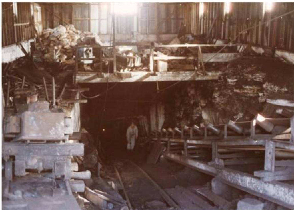
Figure 30. A view down the Sullivan Mine entrance (Feature 23) late in the mine's life, with the rails at centre and conveyor at right. Materials and equipment were stored in the large entrance shed. (Solid Energy, Westport, photo B2020. In Watson and Wright May 2004: plate 29)
