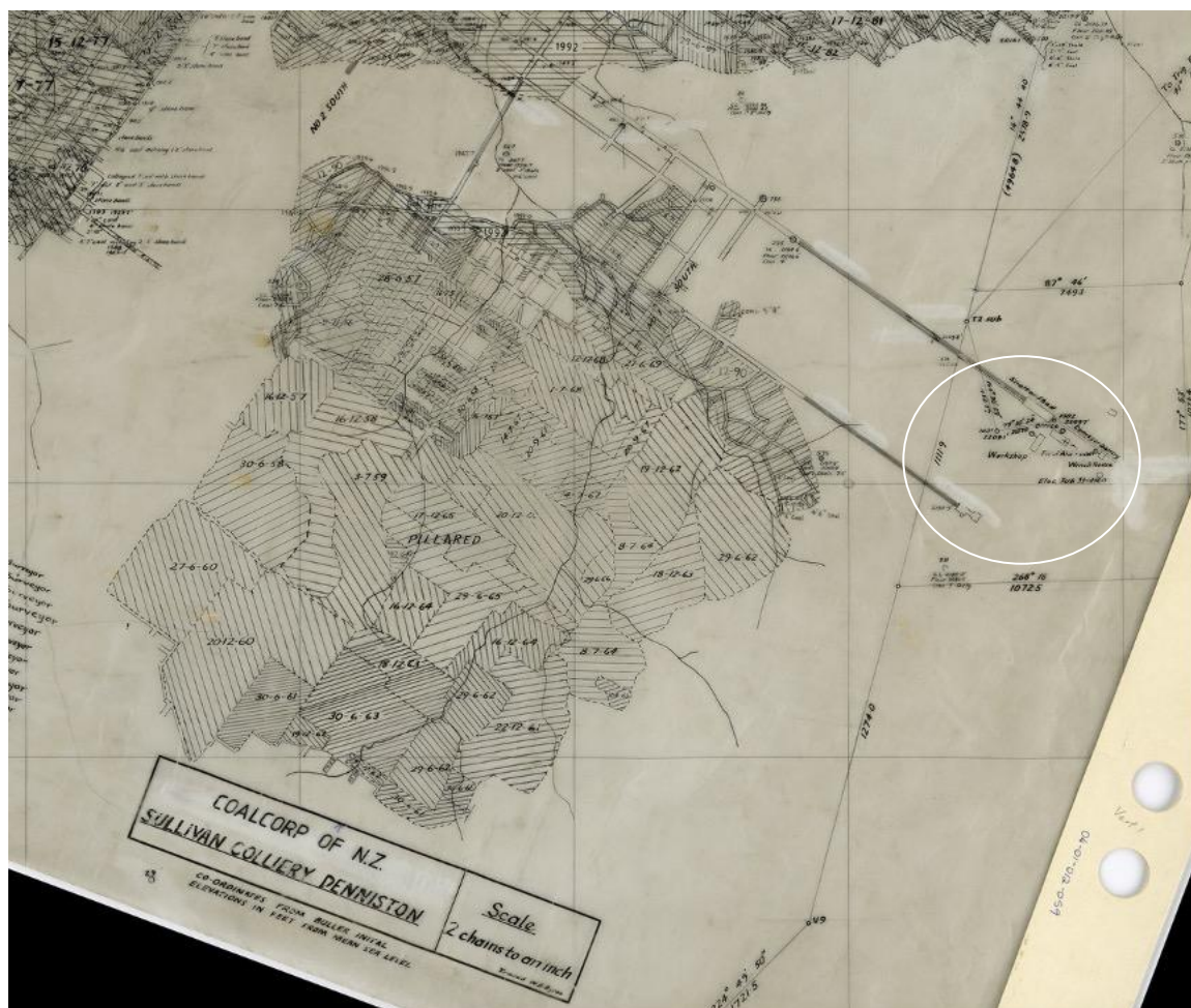
Figure 26. Detail from the Coalcorp of NZ Sullivan Colliery Denniston plan of the No. 1 South Sullivan Mine underground workings. The Sullivan Mine surface features are circled, including the Men and Materials mine entrance and Fan Drift which provided access to the stone drives (source: Bathurst)
