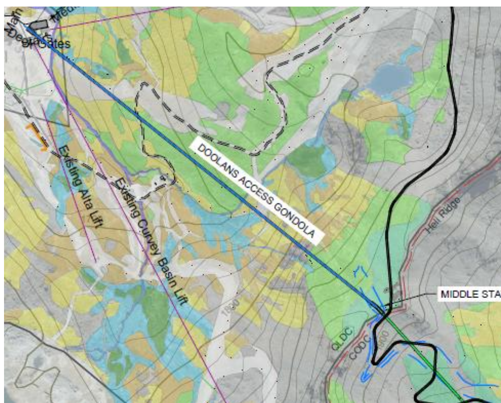
Figure 5.4 – Selected Alignment & Gondola Base Station Location
