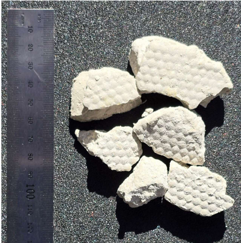
Figure 6: Illustration of Phase 1 sludge (this has been dewatered via pressure filtration). The circular marks are from the sludge pressing against the filter and filter support.
