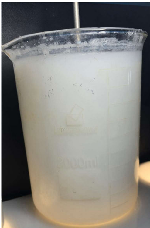
Figure 8: Illustration of Phase 2B sample during flocculation mixing (bright white appearance).
