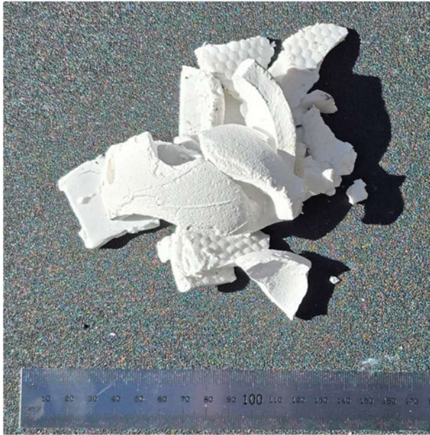
Figure 9: Illustration of Phase 2B sludge – bright white and fine-grained material.
