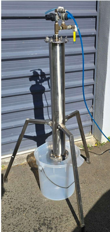
Figure 2: Filtration hardware used on Phase 2B. Filter papers are held on a stainless-steel support base and are clamped into the bottom. Sample is introduced into the top. Air pressure is then set and maintained in the headspace to enhance filtration rates. In this instance dual filters were used.
