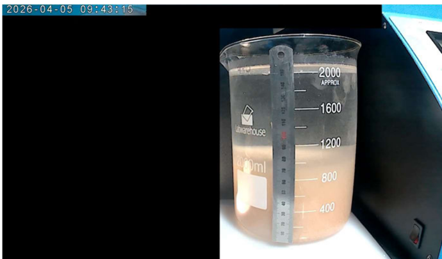
Figure 5: Better view of what Phase 1 sludge looks like (during settle phase). What appears to be iron hydroxide precipitates gives the sludge a light orange, brown colour.
