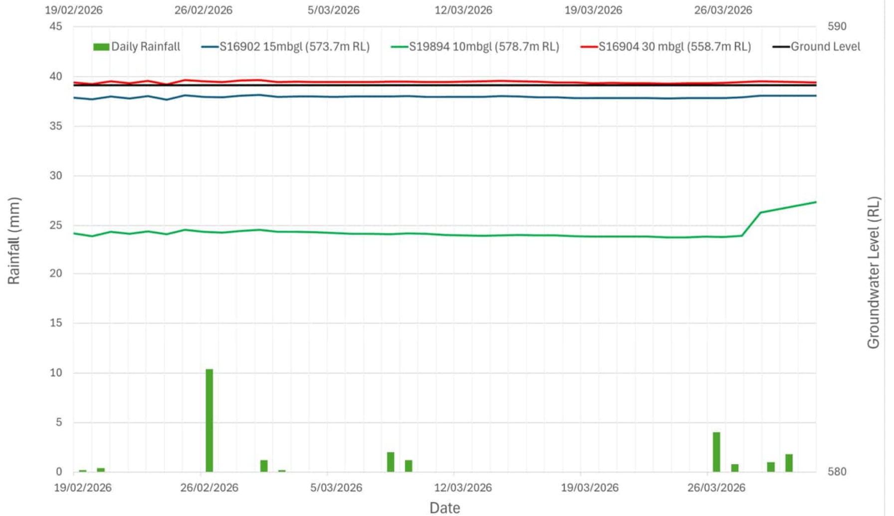
MDD502 - Vibrating Wire Piezometers (19 Feb 2026 to 27 Feb 2026)
