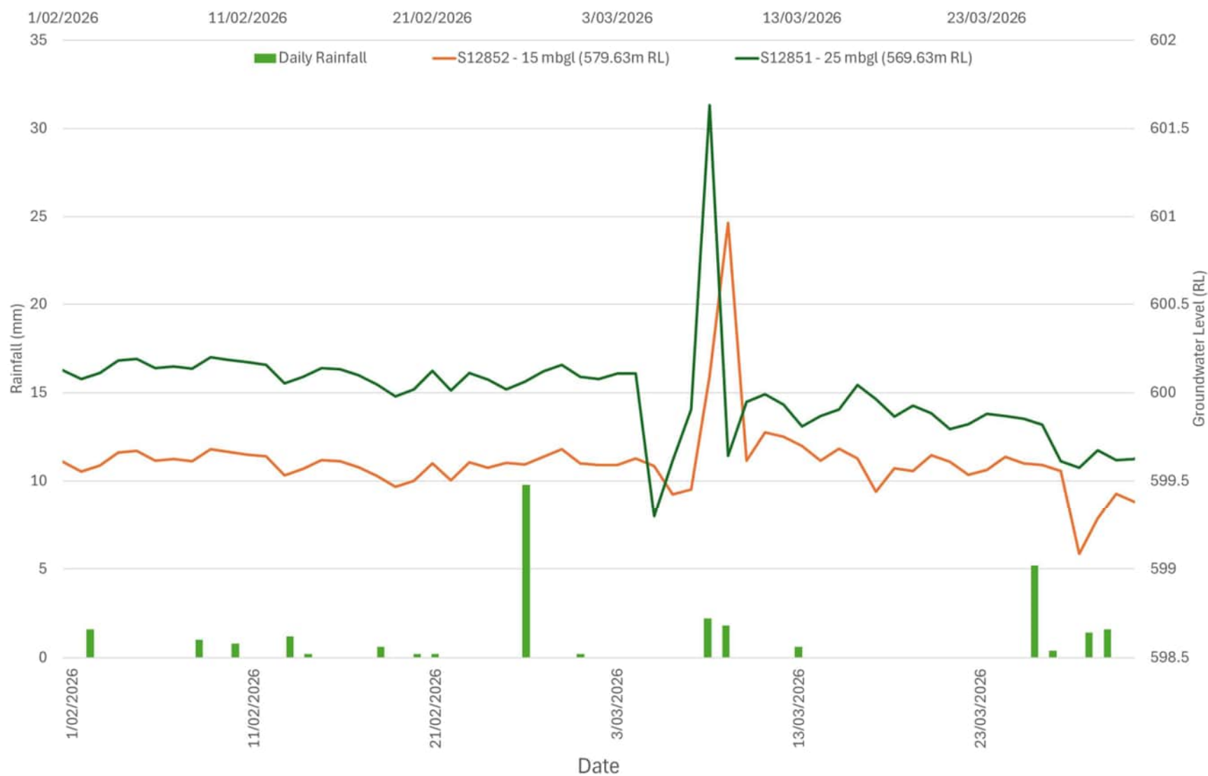
MDD394 - Vibrating Wire Piezometers (01/02/2026 to 31/03/2026)
