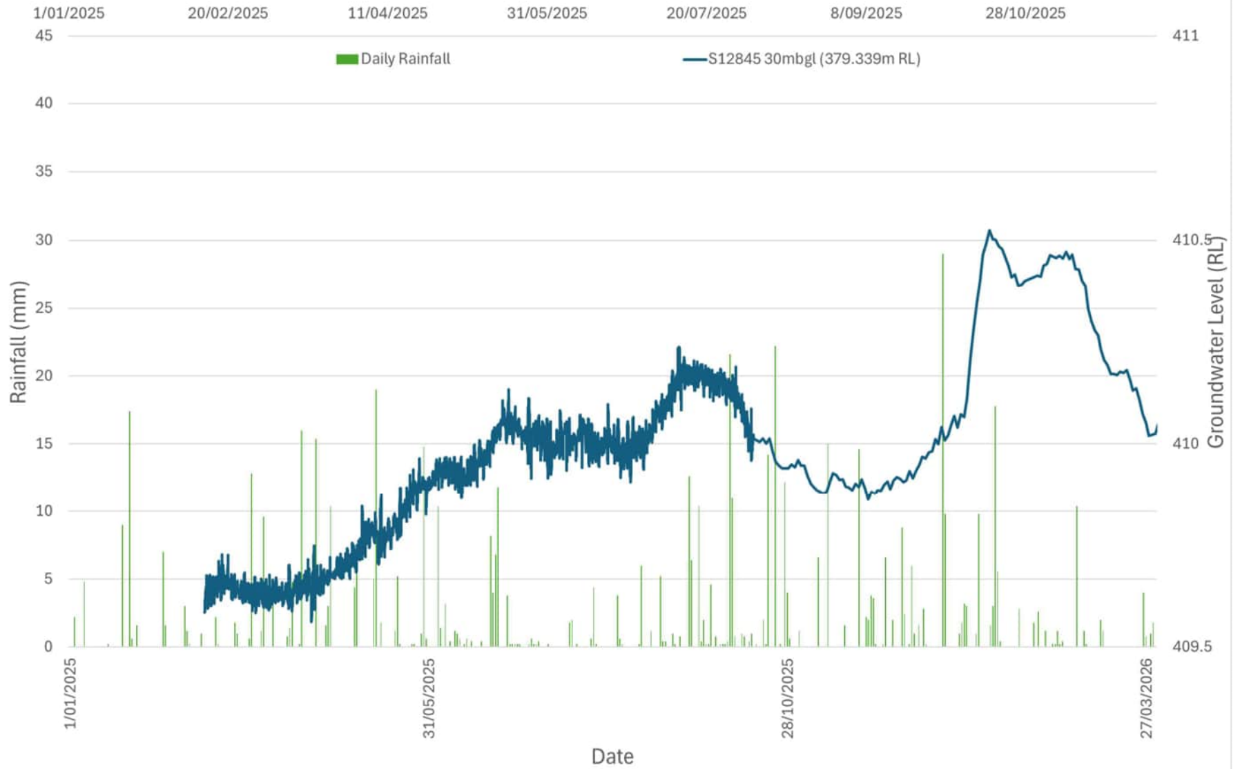
MDD362 - Vibrating Wire Piezometers (1 Jan 2025 to 31 Mar 2026)
