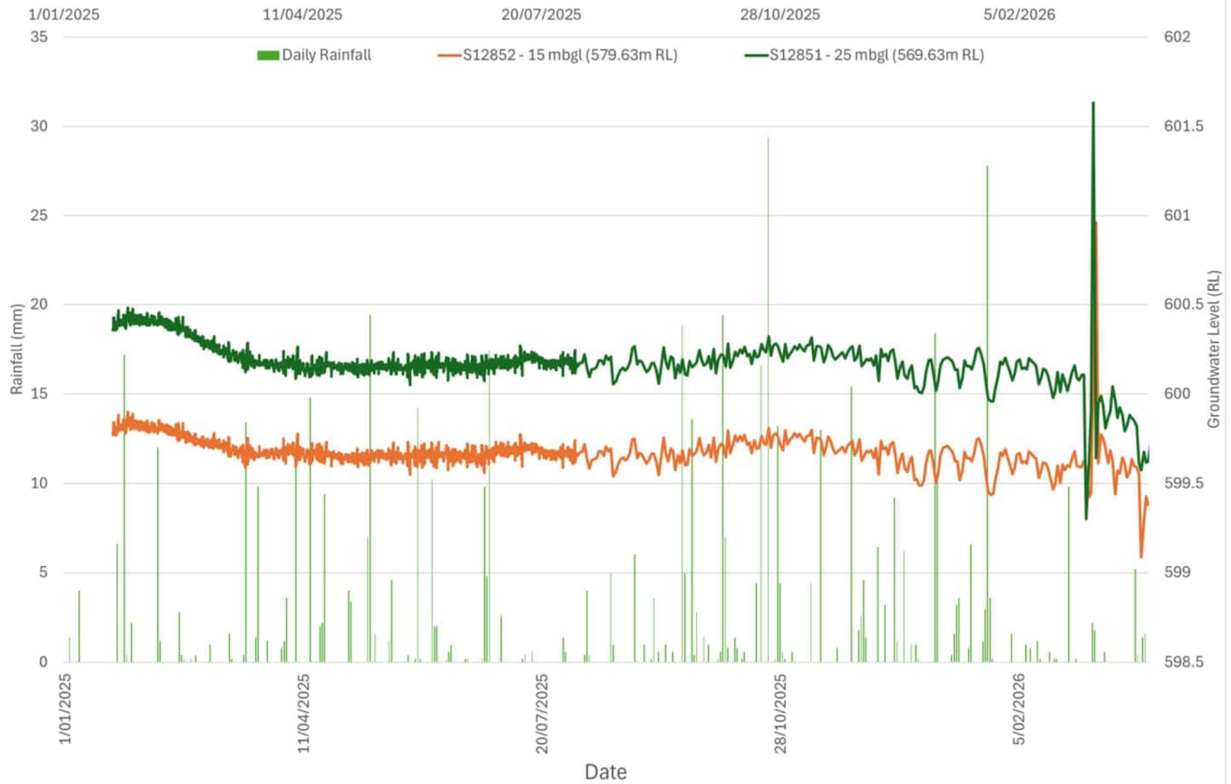
MDD394 - Vibrating Wire Piezometers (01/01/2025 to 31/03/2026)
