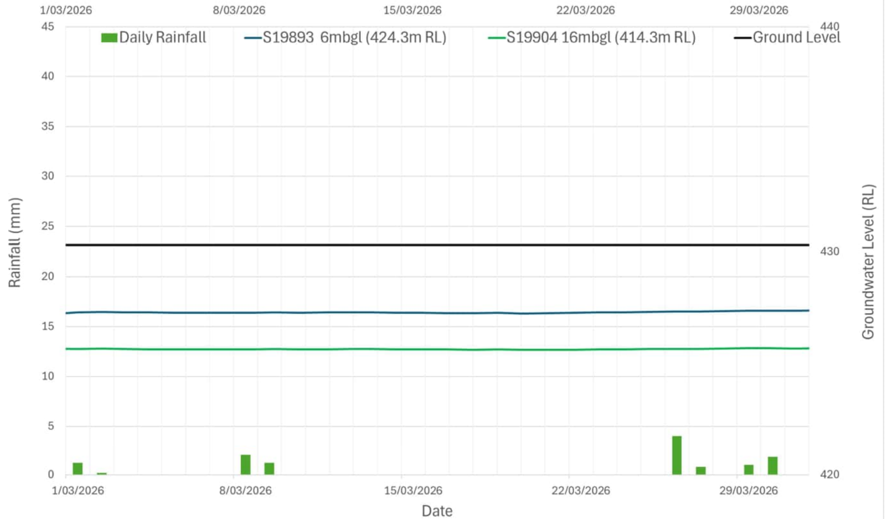
MDD499 - Vibrating Wire Piezometers (1 Mar 2026 to 31 Mar 2026)
