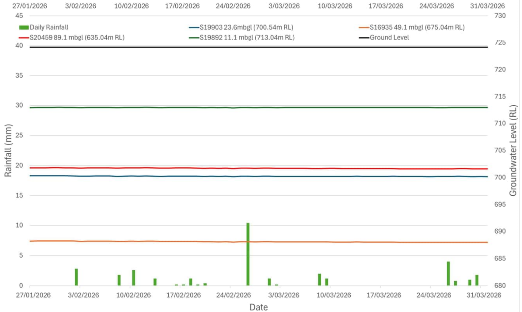
MDD493 - Vibrating Wire Piezometers (27 Jan 2026 to 31 Mar 2026)
