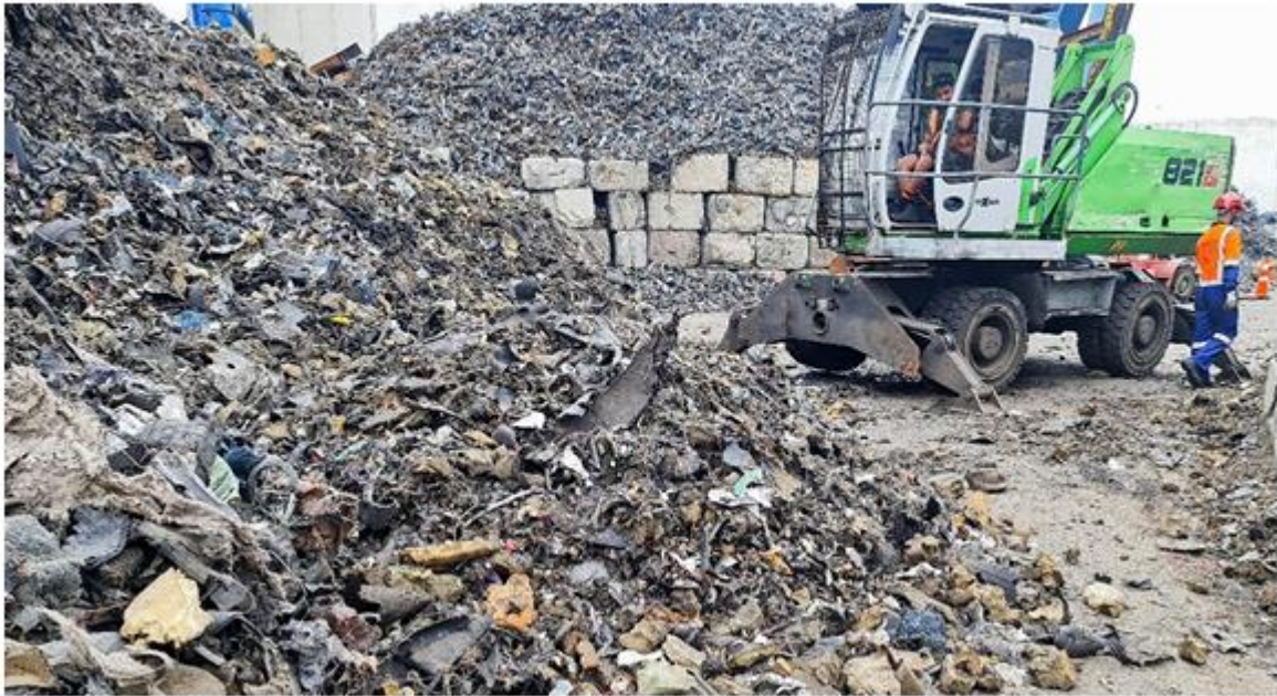
Figure 12 Recovered floc material post-shredding at the process and recovery plant South Auckland
