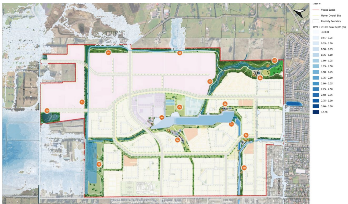
Figure 3 The performance of the proposed stormwater devices intersects with areas identified as open space drainage reserves during a 1:10-year storm event. However, this modelling does not address broader flooding issues across the site that remain unresolved and may further impact the usability of the proposed open space.
