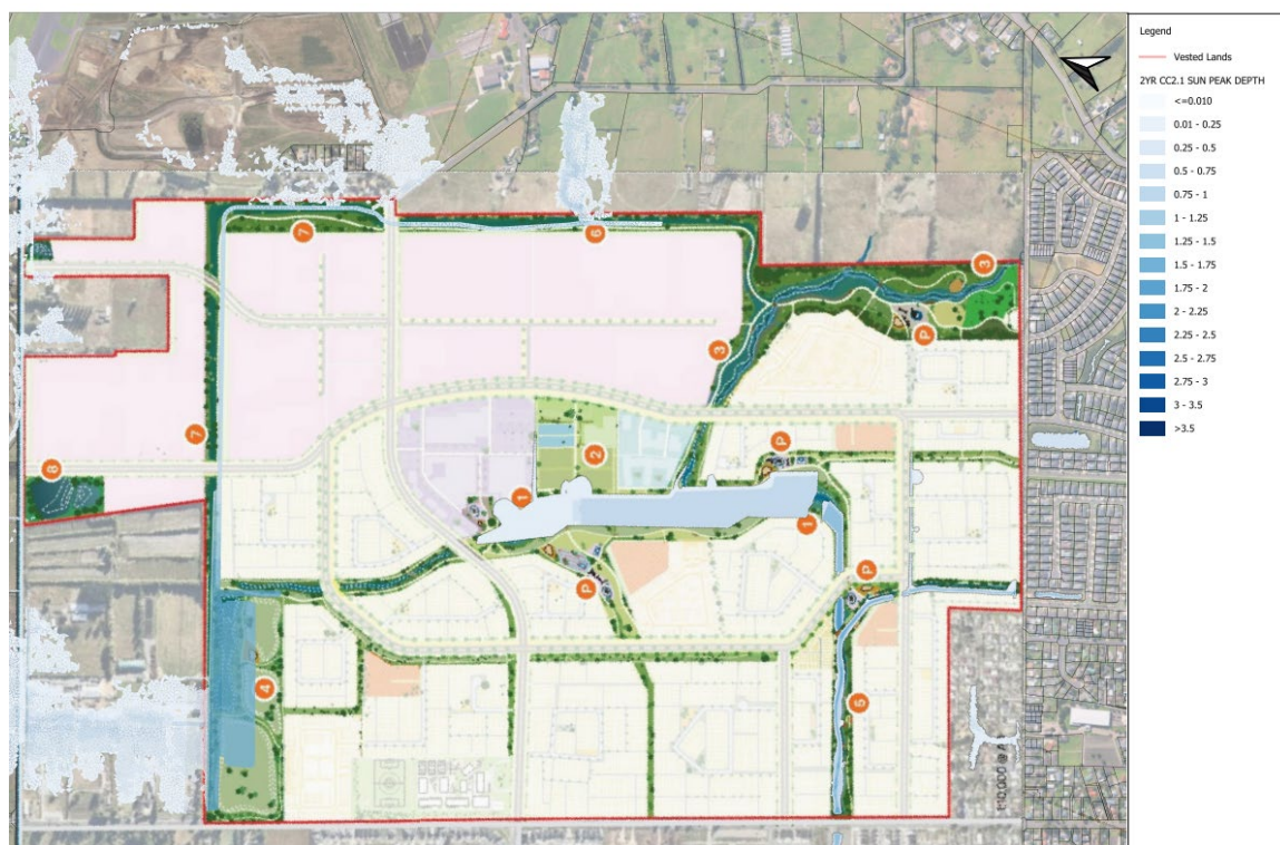
Figure 2 The performance of the proposed stormwater devices intersects with areas identified as open space drainage reserves during a 1:2-year storm event. However, this modelling does not address broader flooding issues across the site that remain unresolved and may further impact the usability of the proposed open space.
