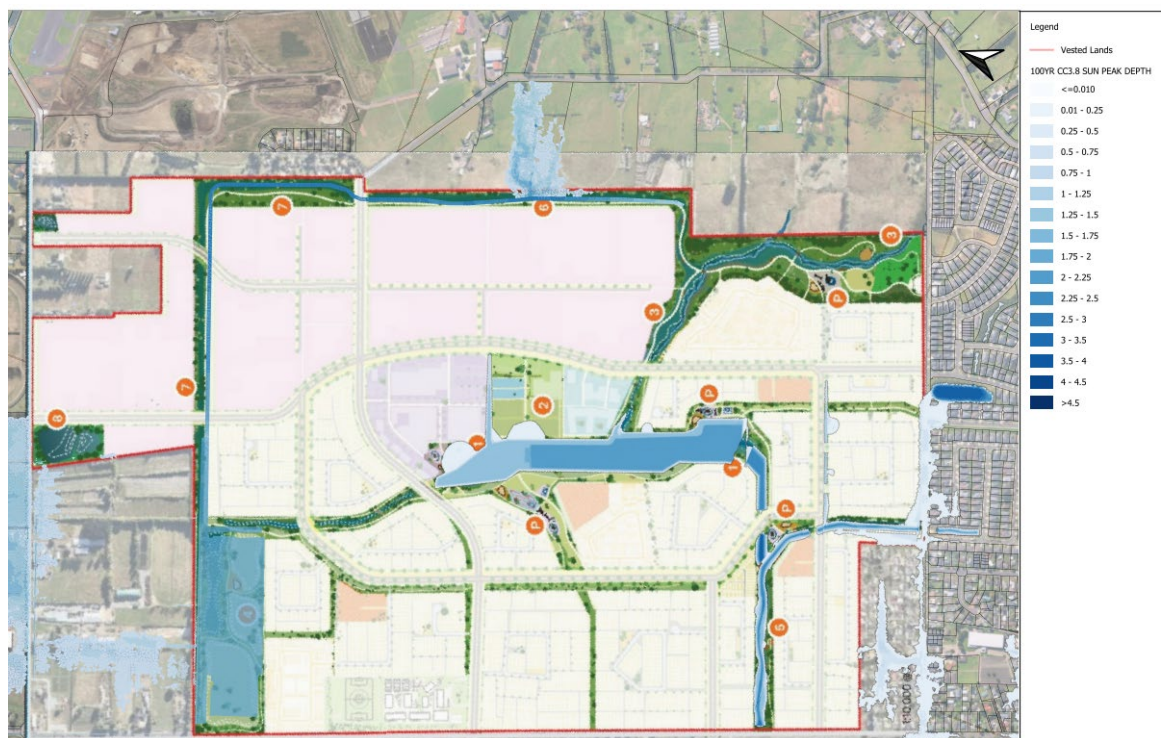
Figure 4 The performance of the proposed stormwater devices intersects with areas identified as open space drainage reserves during a 1:10-year storm event. However, this modelling does not address broader flooding issues across the site that remain unresolved and may further impact the usability of the proposed open space.
