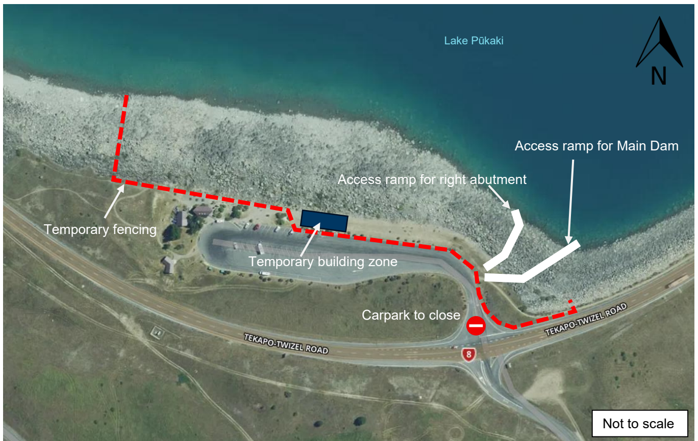
Figure B.2 Dam and right abutment - security fencing, closed access, access ramps and temporary buildings
