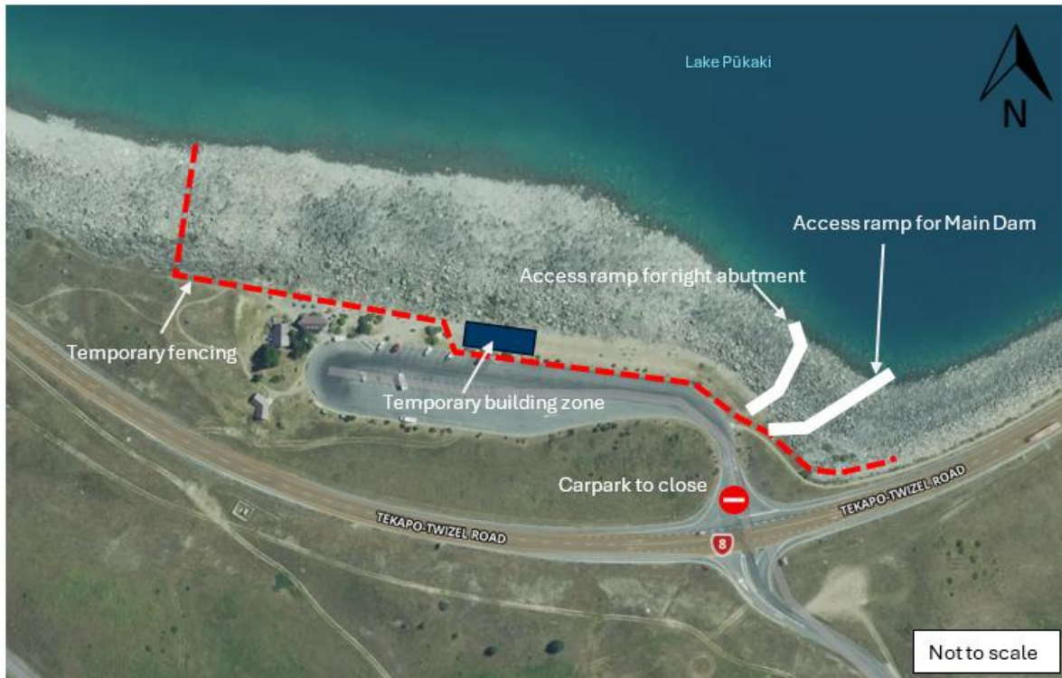
Figure 3 Dam and right abutment - security fencing, closed access, access ramps and temporary buildings
