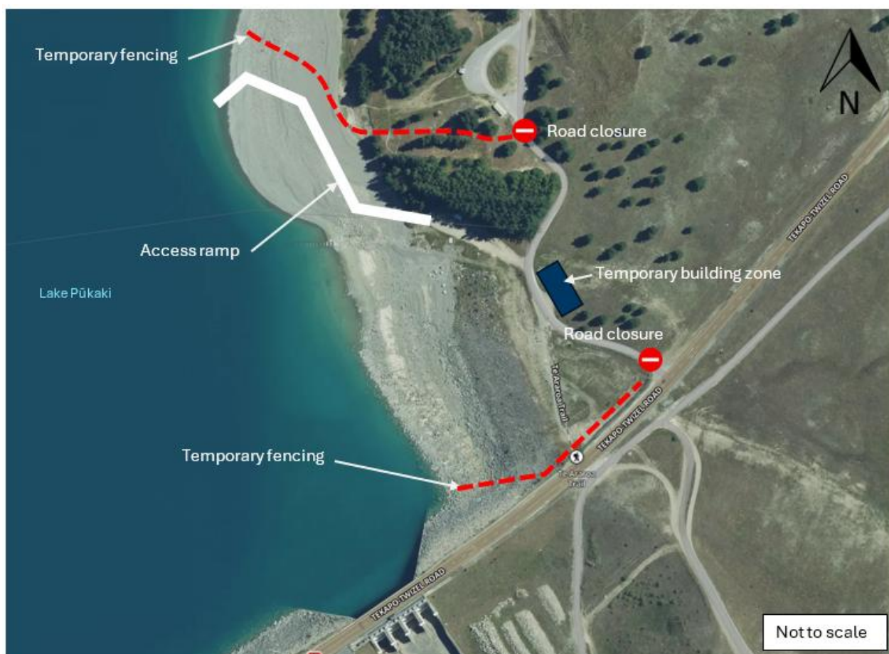
Figure 4 Left abutment - security fencing, closed access and access ramp
